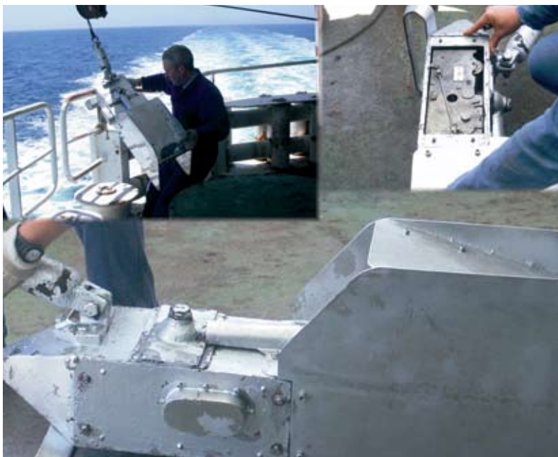
Figure 11: The Continuous Plankton Recorder (CPR). The CPR machines are towed at a depth of about 7 metres along regular routes at monthly intervals. The CPR works by filtering plankton from seawater over long distances (up to 500 nautical miles) on a moving filter band of silk. The filter silk band is wound through the CPR on rollers and stored on a cassette until analysed in the laboratory.
