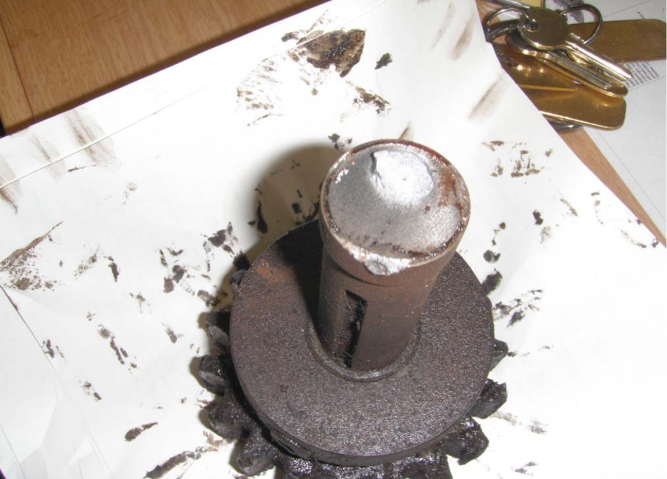
Gearwheel and shaft showing shear plane:
