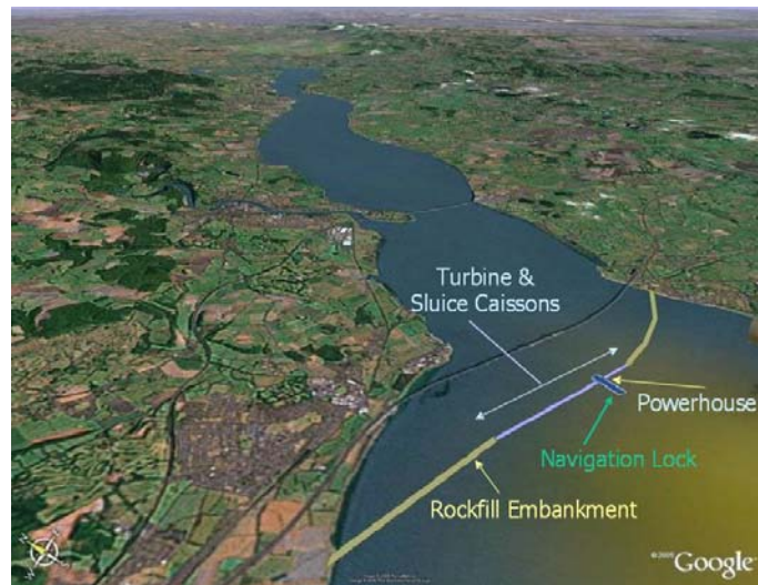
Figure 3. An aerial view of the proposed Shoots Barrage (from Parsons Brinckerhoff, Underlying image from Google Earth).
