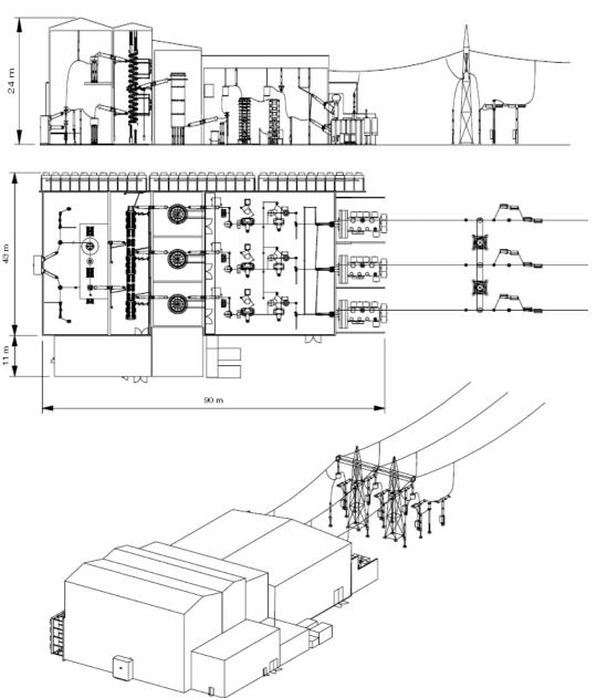
Figure A1-18: Indicative dimensions of a Voltage Source Converter (VSC) High Voltage Direct Current (HVDC) Converter Station (Example: HVDC Light © ABB)
