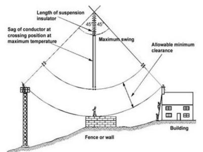
Figure A1-28 Safety Clearance to Objects (on which a person can stand)
