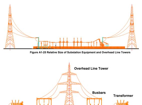
Figure A1-26 Relative Size of Substation Equipment and Overhead Line Towers
