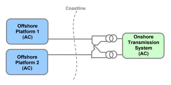
Figure A1-16: Assumed Sharing of Assets forming part of the Offshore Transmission System
