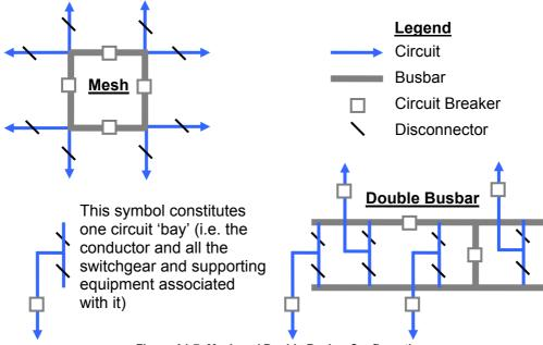
Figure A1-7: Mesh and Double Busbar Configurations
