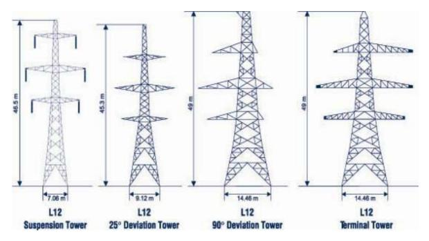
Figure A1-24: Typical Towers in a 400kV Route (L12 example)
