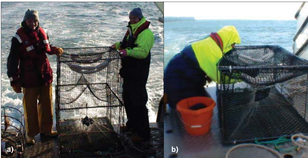
Figure 24: a) The fish trap extended into upper and lower parlours as it would sit on the seabed. b) Trap with the upper parlour collapsed showing the support frames added to hold the entrance open in the strong tidal currents experienced along the north Yorkshire coast.
