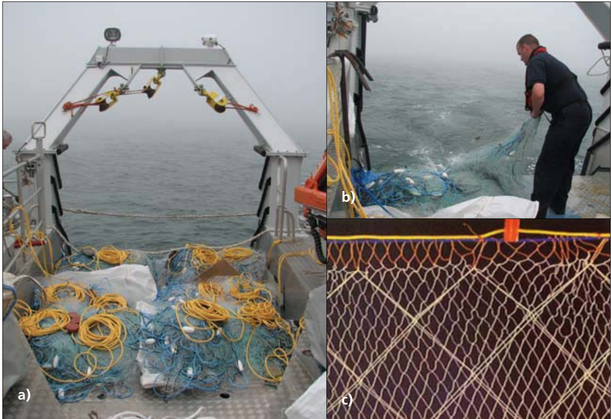
Figure 25: a) Six fleets of trammel net ready to deploy on the aft deck of North Eastern Guardian III . b) Deploying a fleet of trammel net. c) The construction of a trammel net.
