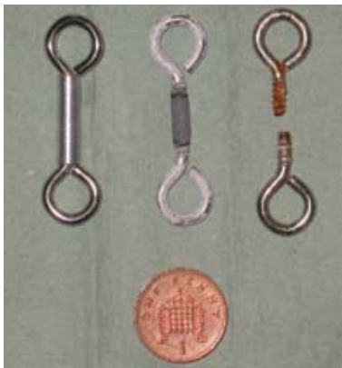
Figure 27: The decay of the galvanic mechanism timed to release juvenile lobsters within 48 hours (with 1p coin for scale)
