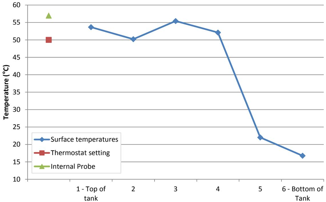
Figure 26: Temperature profile of 150litre cylinder when heated to 50°C at the start of the test
