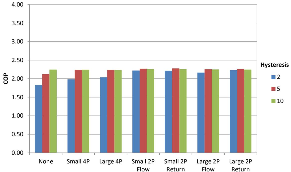
Figure 46: Effect of different configurations and hysteresis on COP for an ASHP with 4 rads
