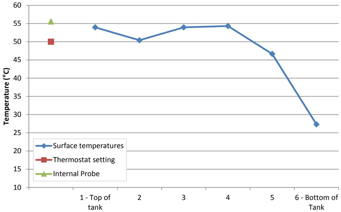
Figure 27: Temperature profile of 250litre cylinder when heated to 50°C
