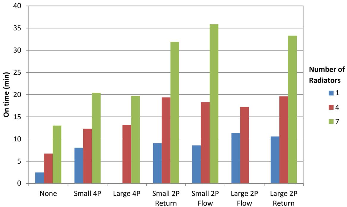
**Figure 43: Effect of system size and configuration on on-time for different numbers of radiators with a hysteresis of 5°C**
