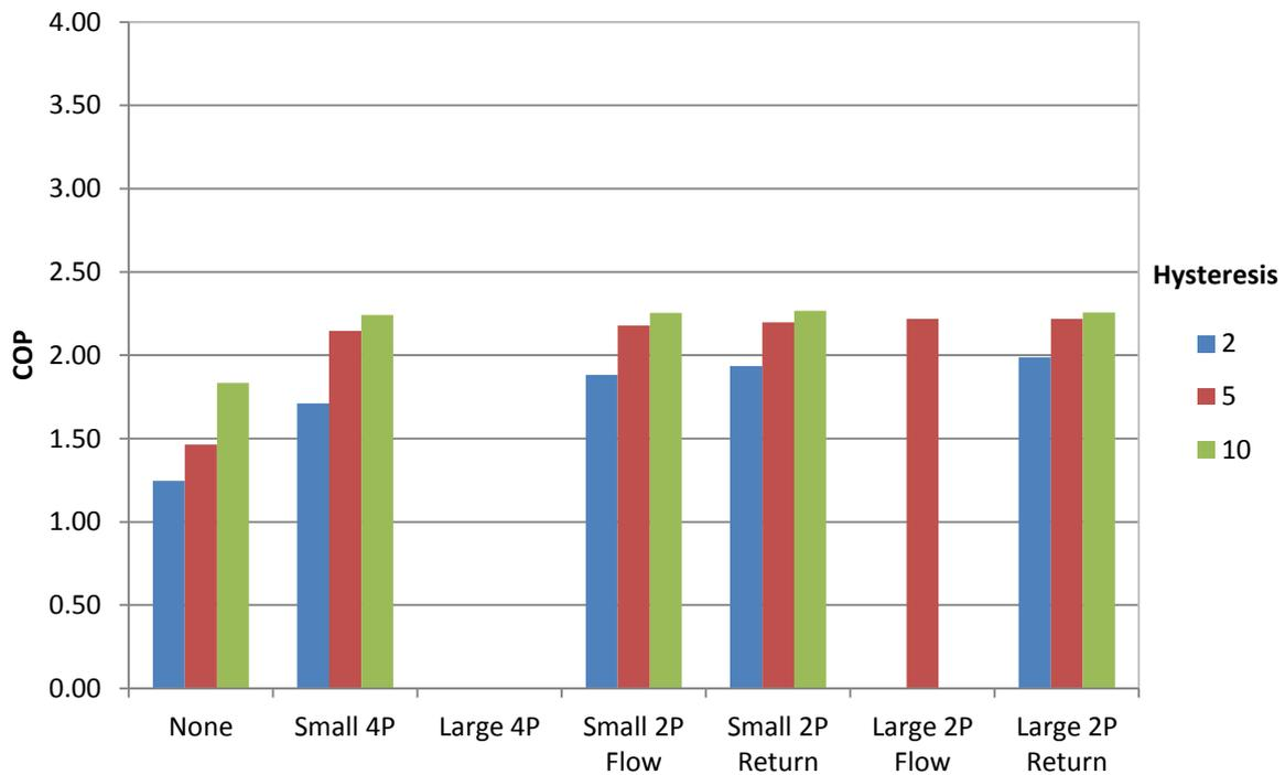
Figure 48: Effect of different configurations and hysteresis on COP for an ASHP with 1 rad
