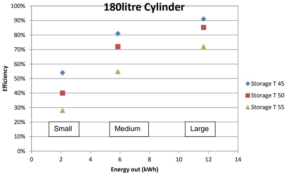
Figure 14: Efficiency at different storage temperatures and draw-off patterns for 180litre cylinder
