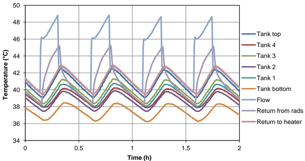
**Figure 39: Stratification of the 90litre tank in the return configuration**
