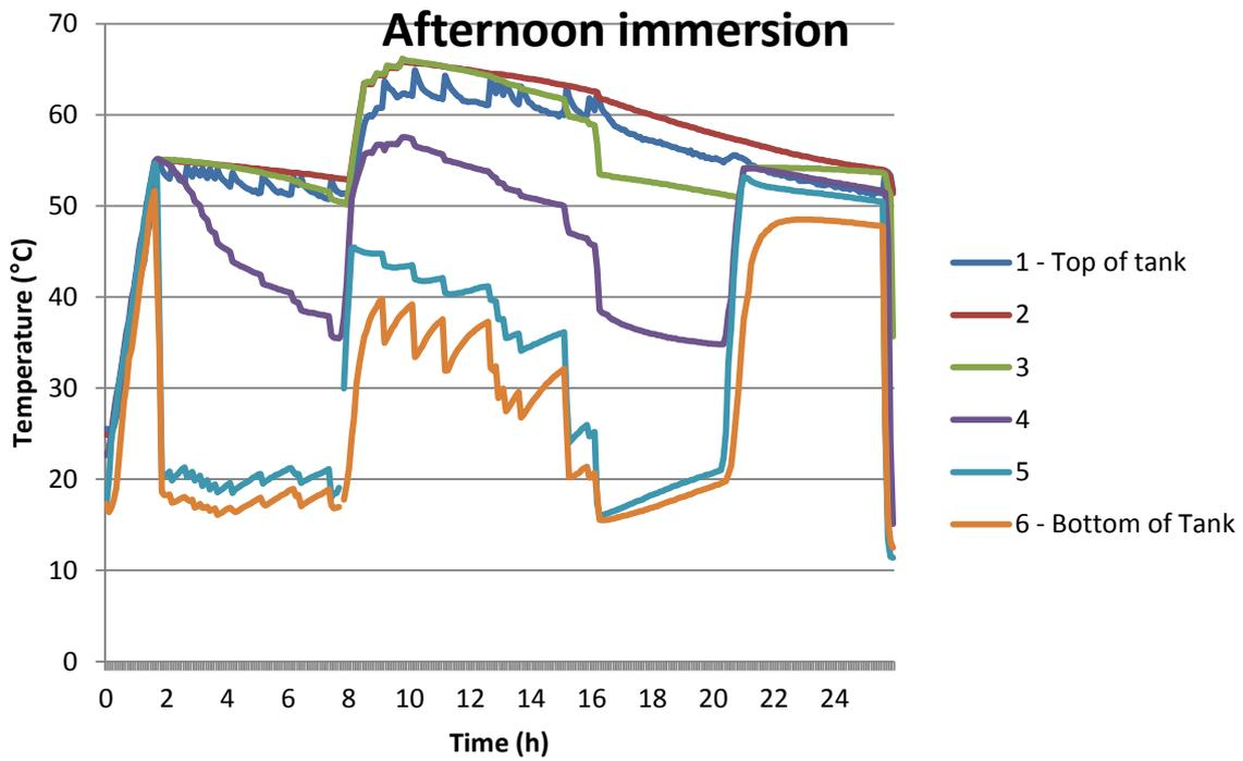
Figure 23: Temperature profile when using immersion at lunchtime
