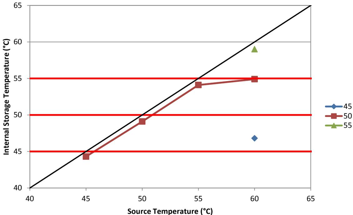
**Figure 18: Source temperature compared to set point and actual storage temperature**
