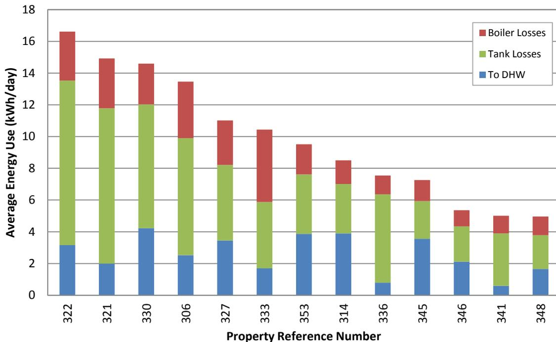
Figure 2: Distribution of energy losses from system boilers
