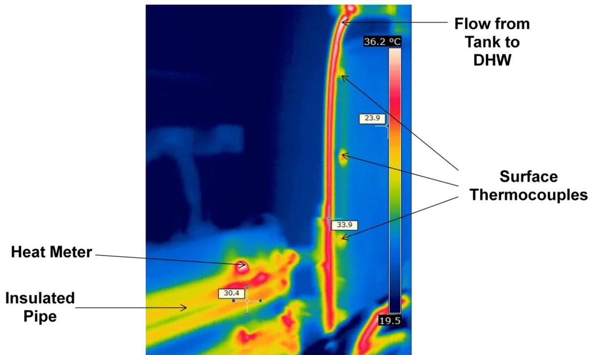
Figure 29: Thermogram of 180litre cylinder
