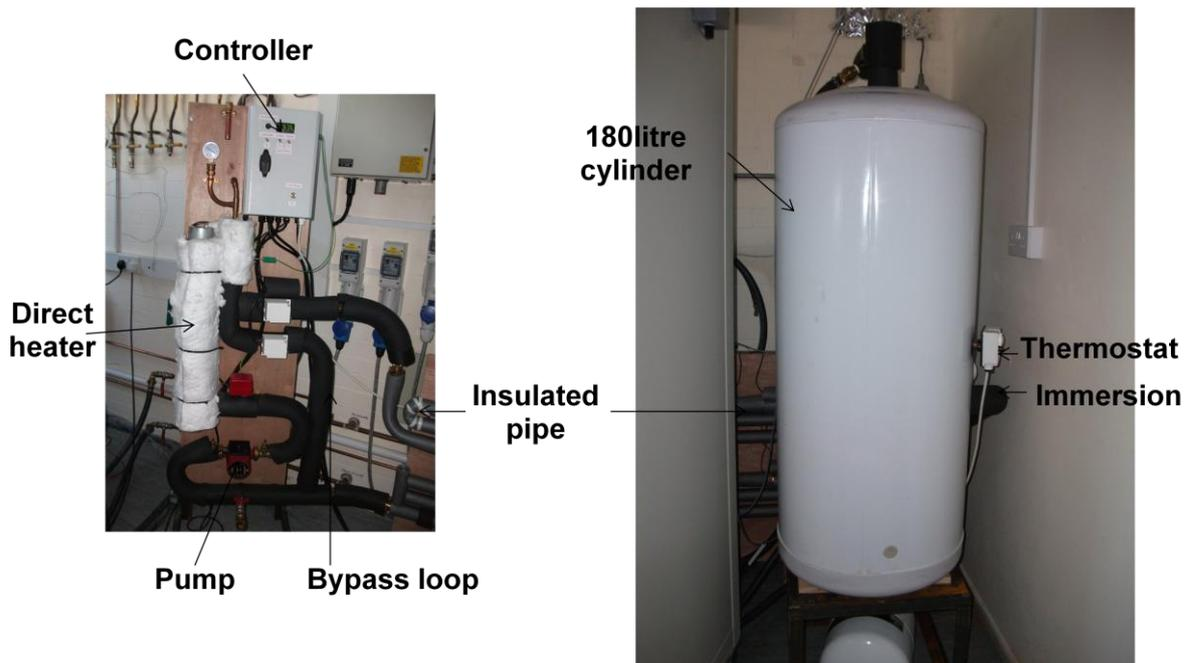
**Figure 11: Modified section of test rig including direct heater, 180litre cylinder on test rig**
