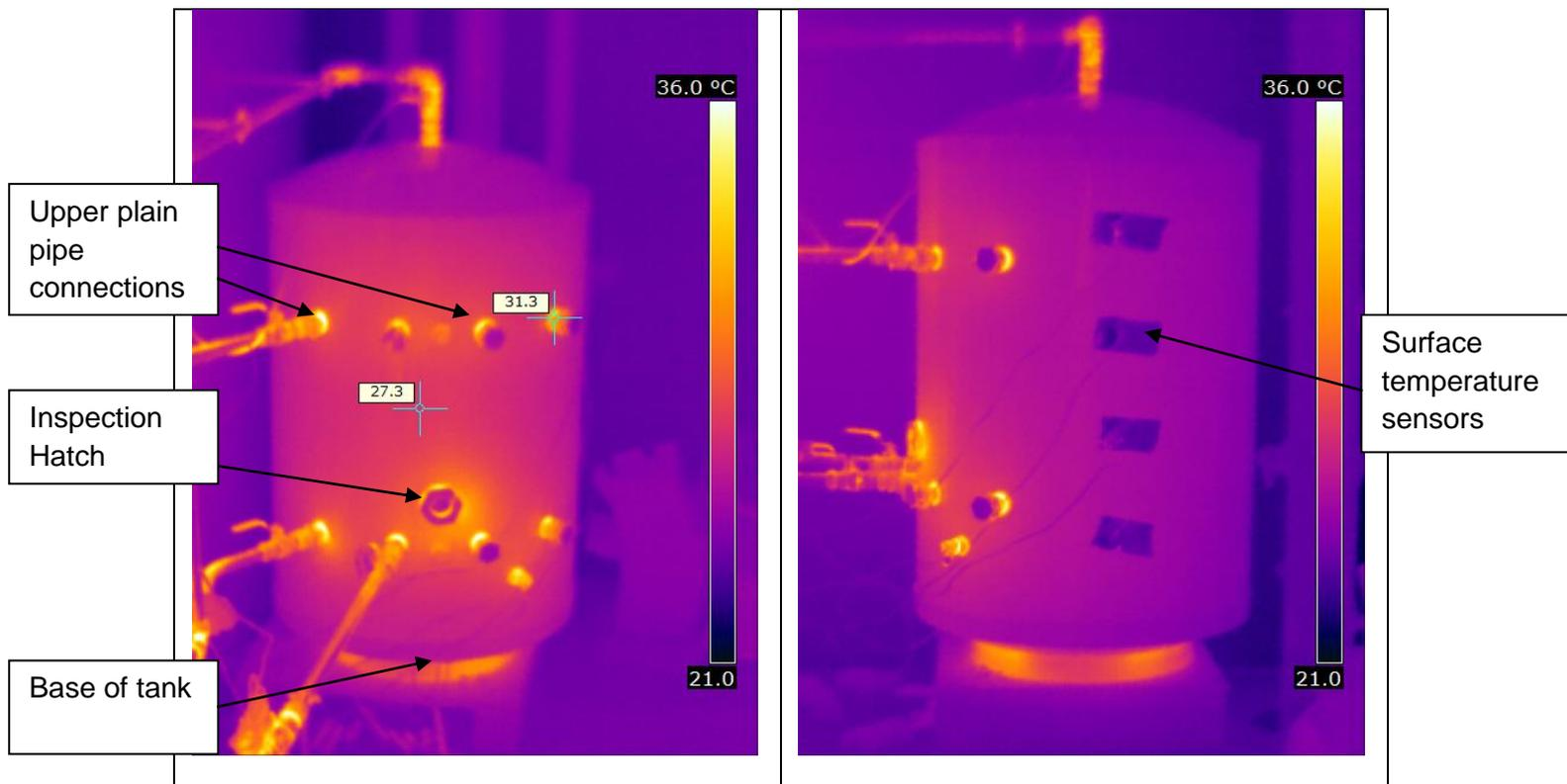
Figure 37: Thermal images of the buffer tank
