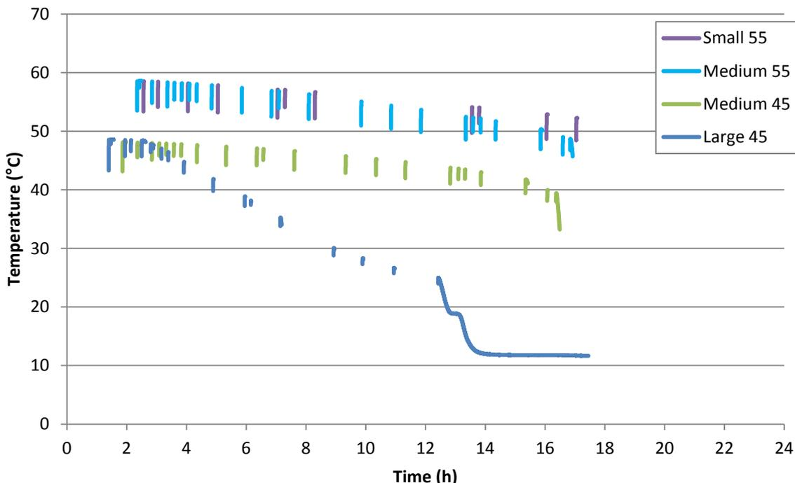
**Figure 20: Exit temperature of water from cylinder during off-peak tests**
