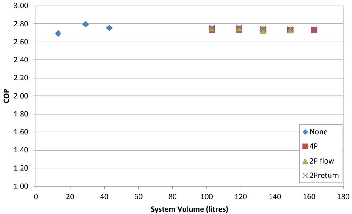
Figure 49: Effect of system volume on COP for ground source heat pumps
