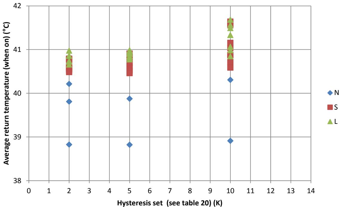
**Figure 41: Average return temperature when the system is in operation for different configurations N = no buffer tank, S = small buffer tank and L = large buffer tank.**
