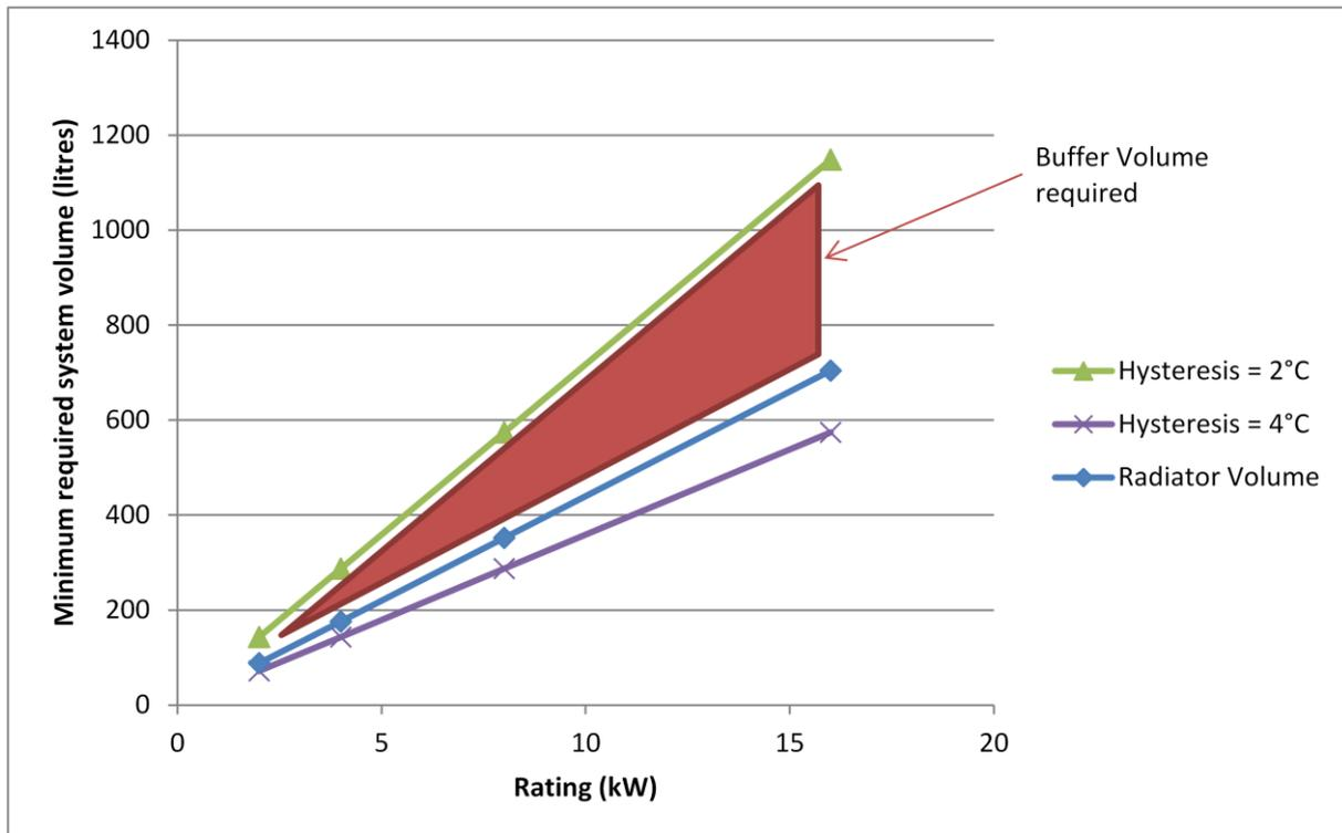
**Figure 51: Minimum system volume for different hysteresis at different rated outputs**
