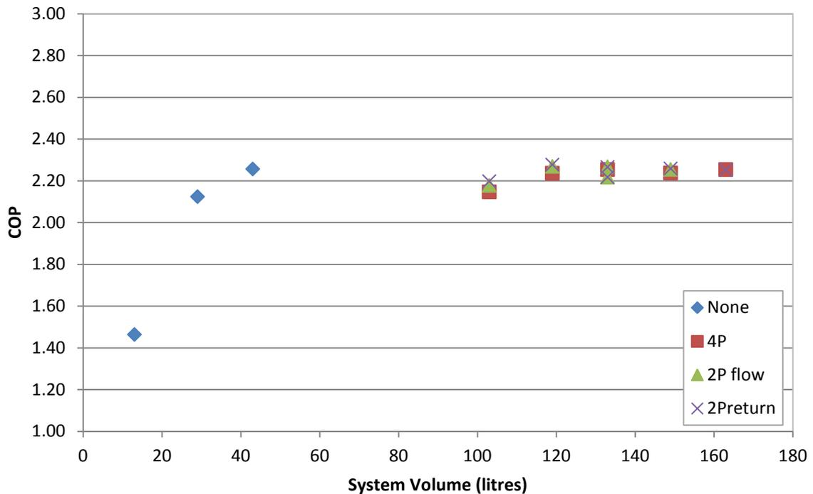
Figure 50: Effect of system volume on COP for air source heat pumps
