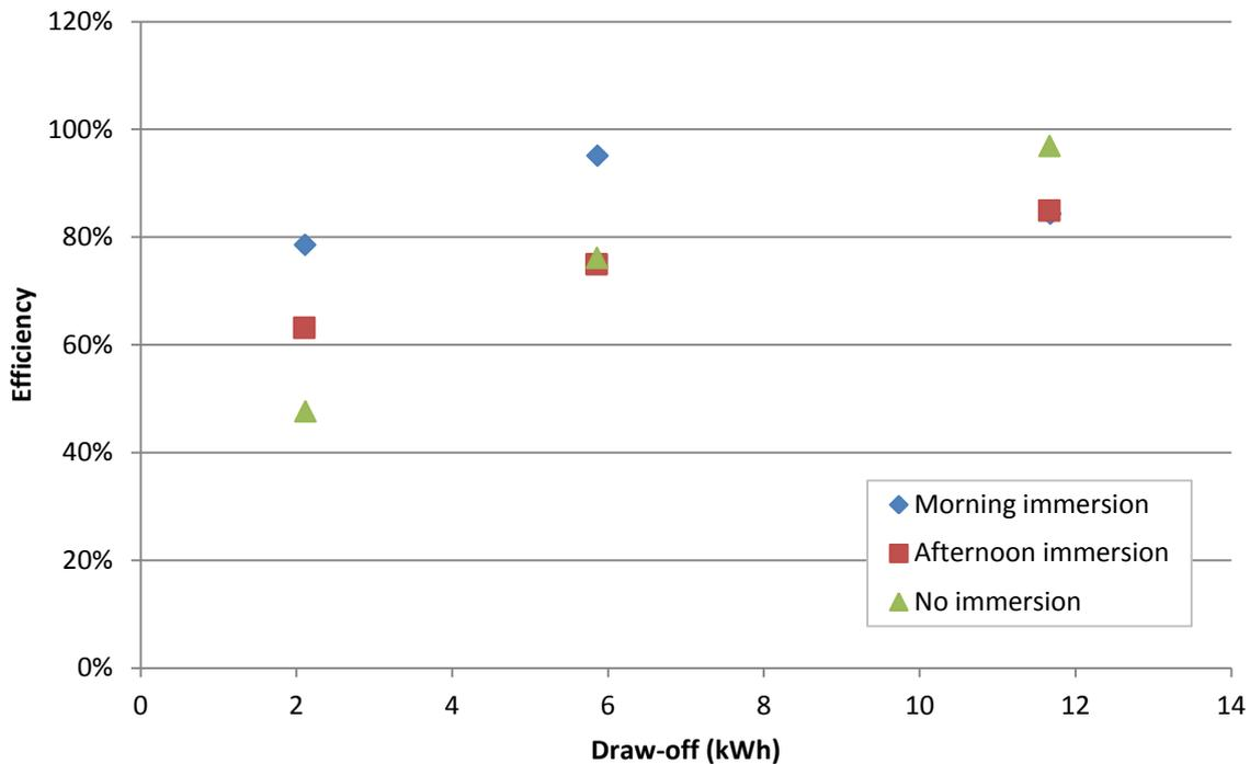
**Figure 22: Effect of immersion on efficiency**
