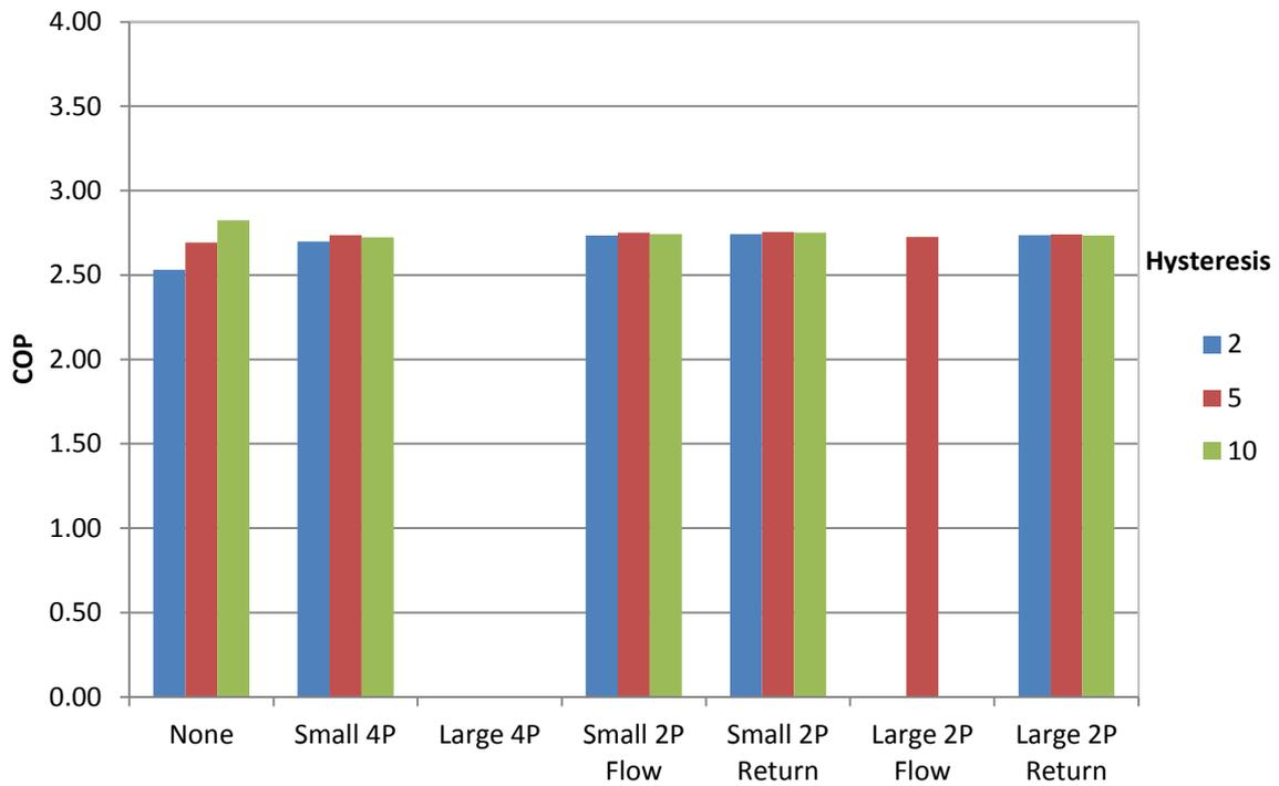
Figure 47: Effect of different configurations and hysteresis on COP for a GSHP with 1 rad
