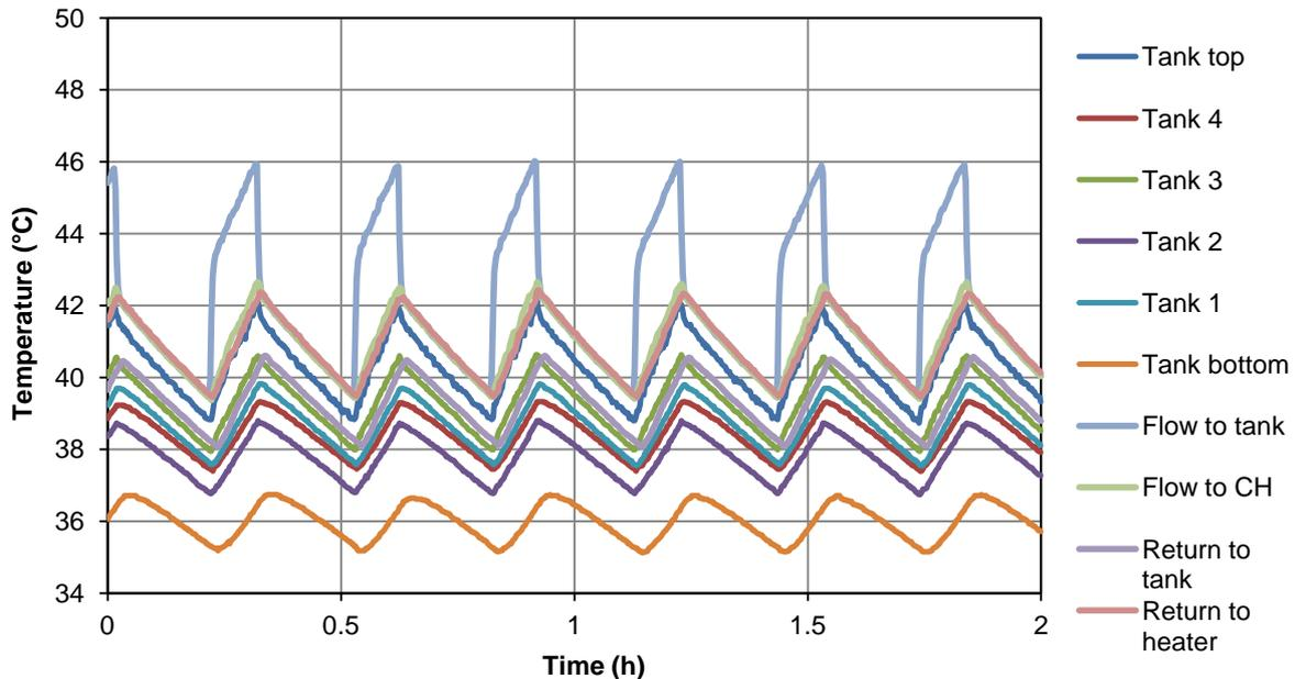
**Figure 40: Stratification of the 90litre tank in the 4 pipe configuration**
