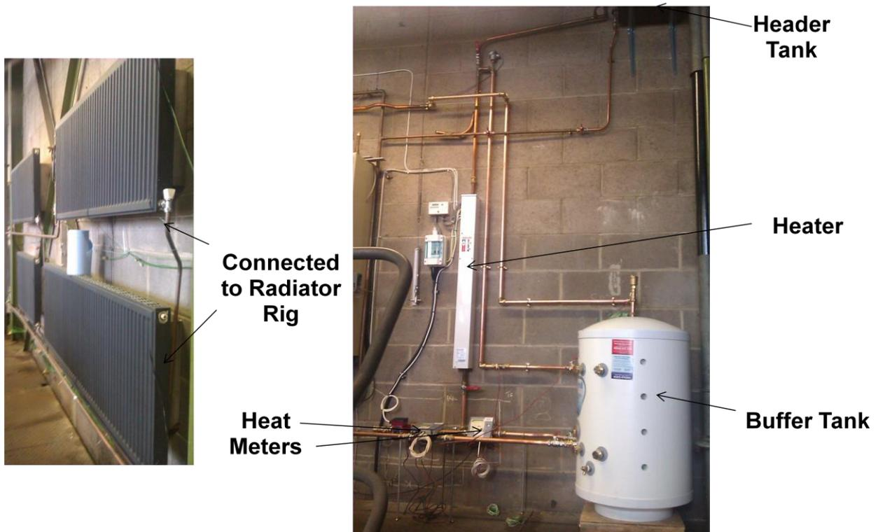
**Figure 33: Buffer tank test rig at Kiwa**
