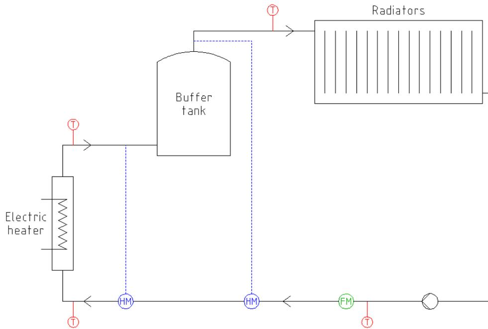
**Figure 35: 2 pipe in the flow from the heater**
