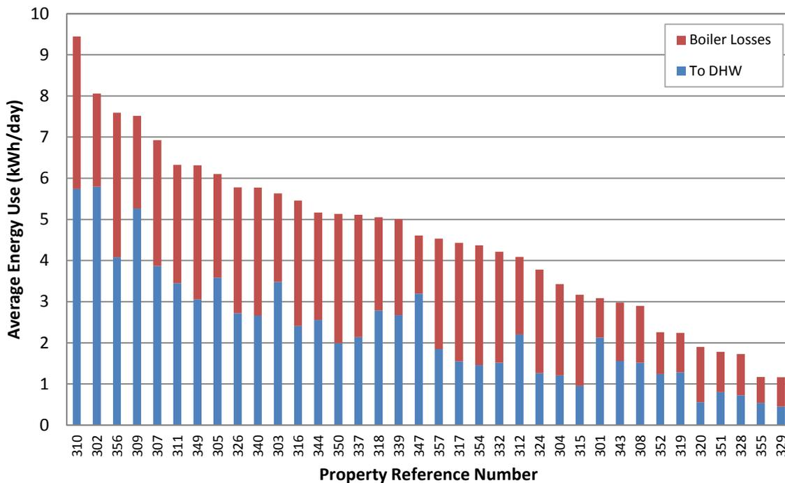
**Figure 5: Combi boiler losses compared to DHW output**
