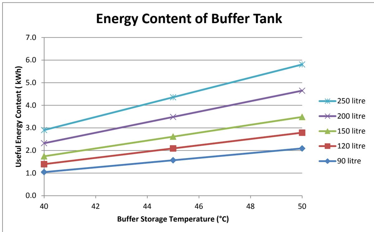
Figure 52: Energy content above 30°C of buffer tanks
