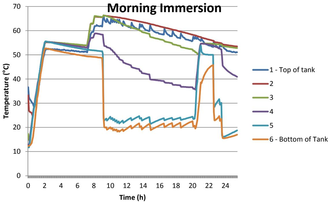
Figure 24: Temperature profile when using immersion in the morning
