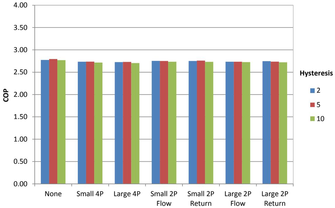
Figure 45: Effect of different configurations and hysteresis on COP for a GSHP with 4 rads
