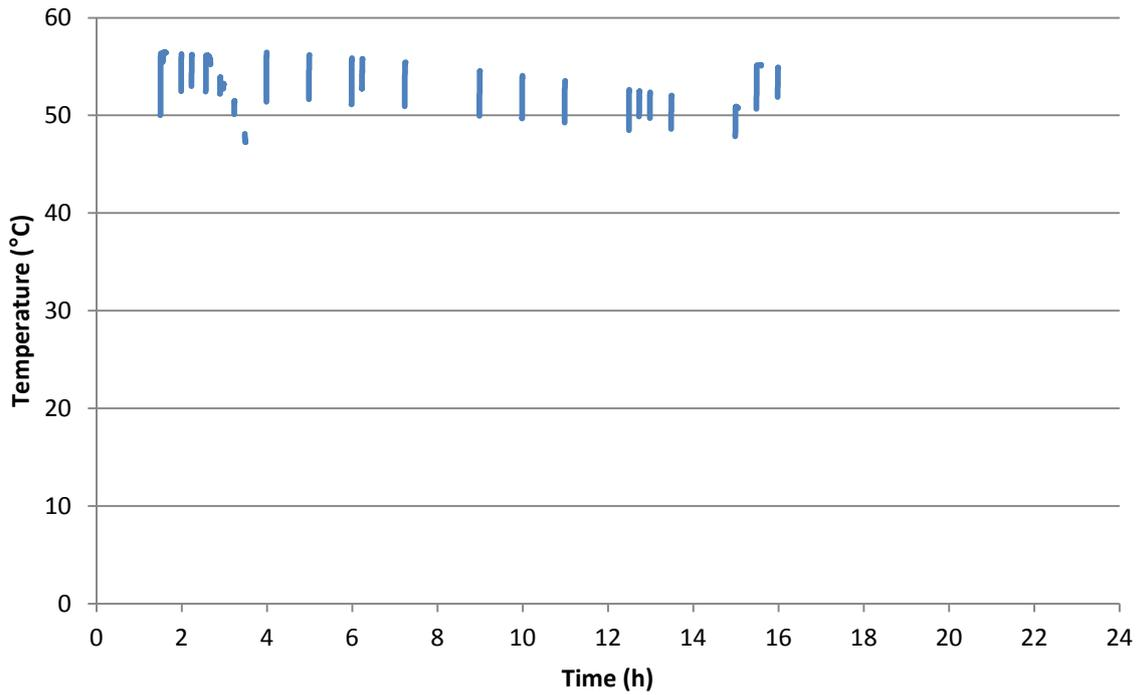
Figure 25: Water exit temperature from the 150litre cylinder in the large draw-off pattern (only when there is a flow)
