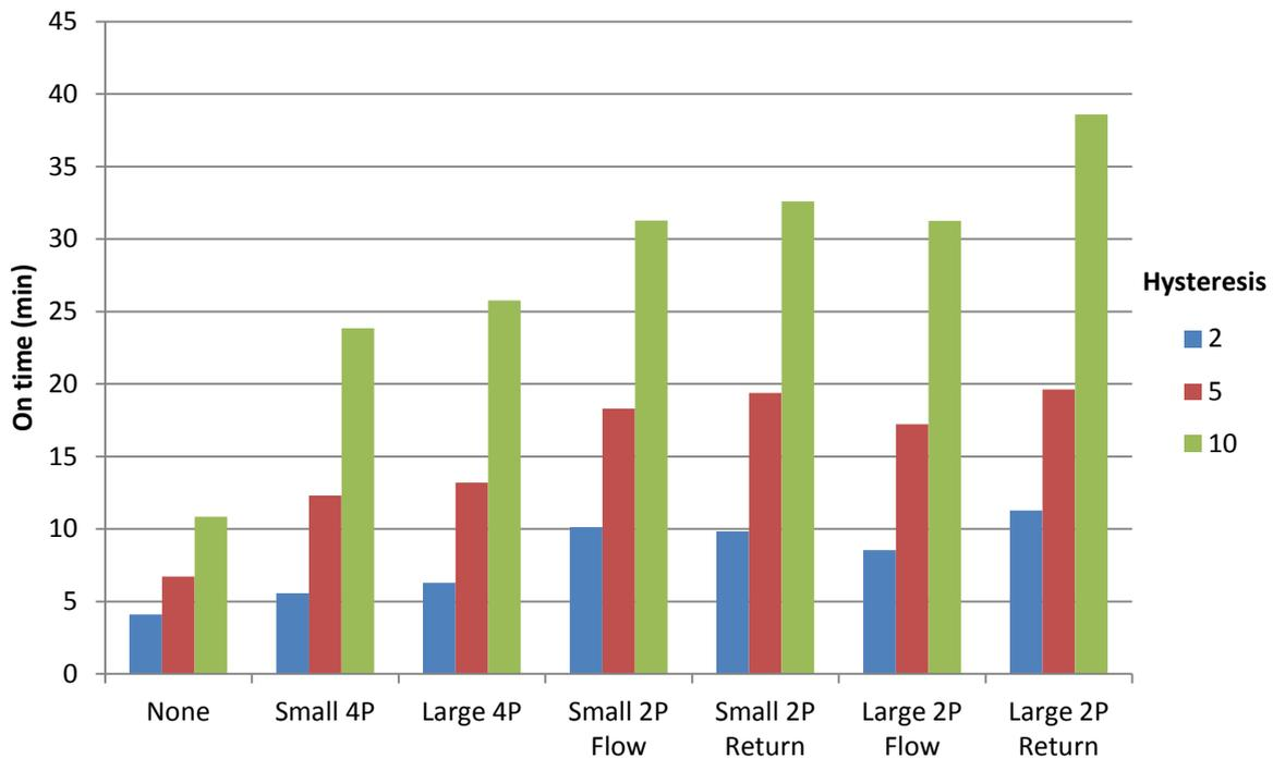
**Figure 42: On time with 4 radiators showing the effect of hysteresis and different configurations**
