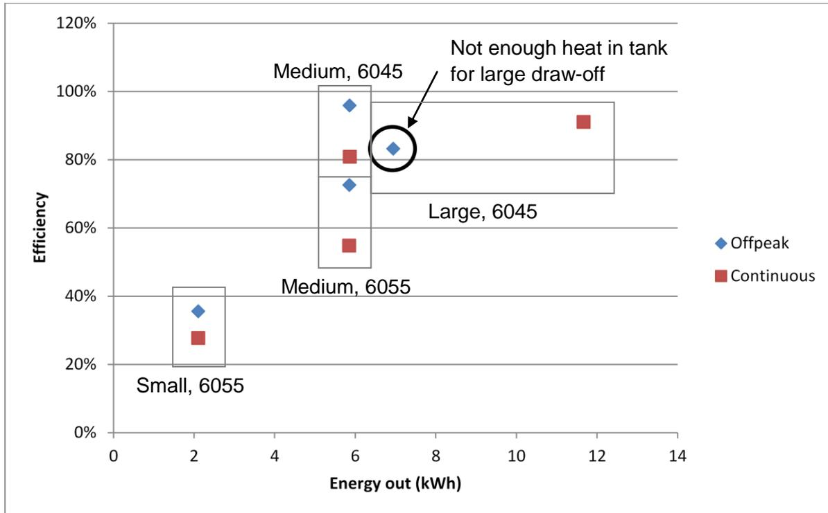
Figure 19: Off-peak vs. continuous heating and the effect on efficiency
