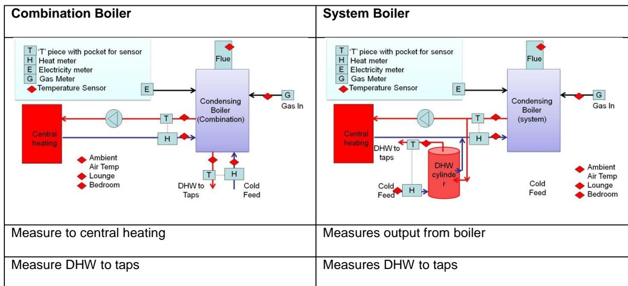
Figure 1: Measurement configurations for combination and system boilers
