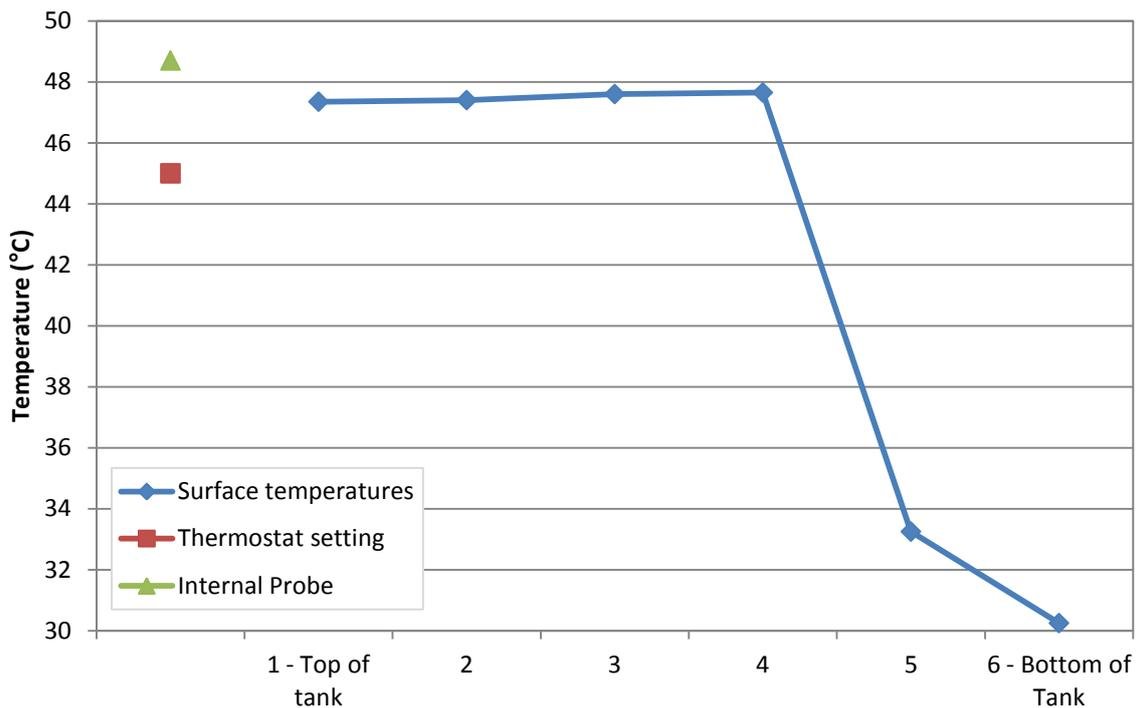
Figure 13: Temperature profile of 180litre cylinder when heated to 45°C at the start of the test
