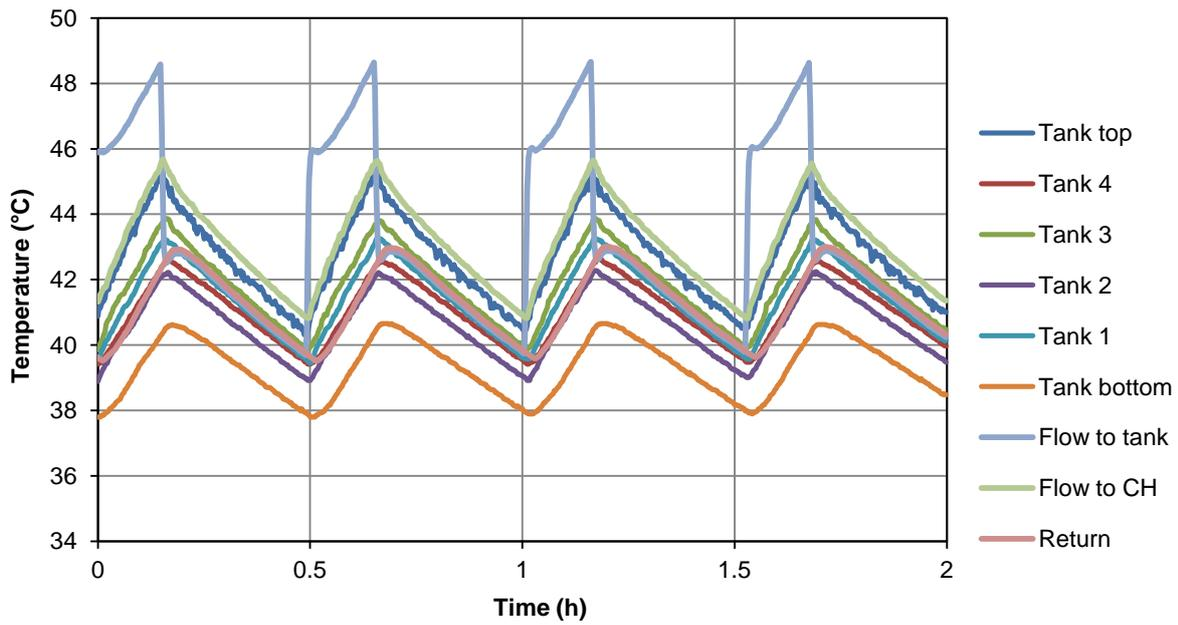
**Figure 38: Stratification of the 90litre tank in the flow configuration**
