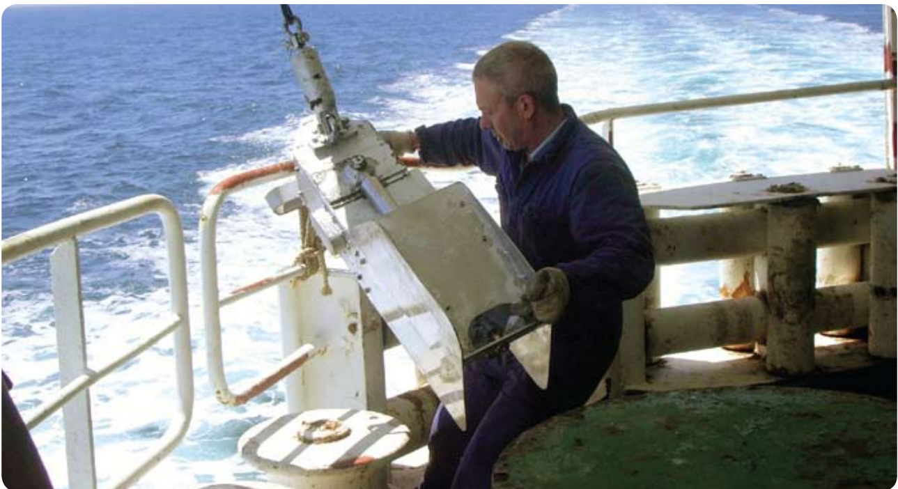
SAHFOS' Continuous Plankton Recorder being deployed from the P&O Ferries' Pride of Bilbao
