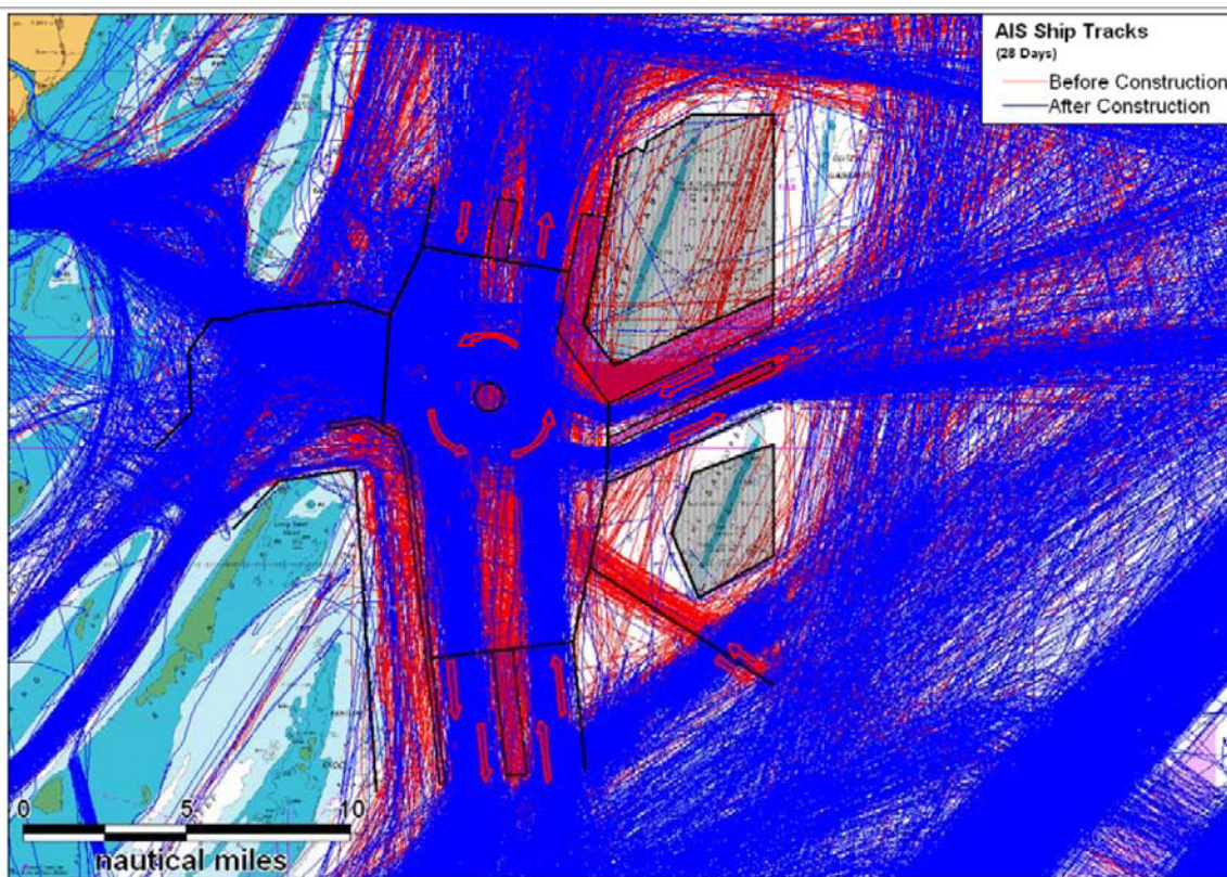
Figure 5.31 - AIS ship tracks before and after the construction of the Greater Gabbard wind farm and traffic separation scheme
