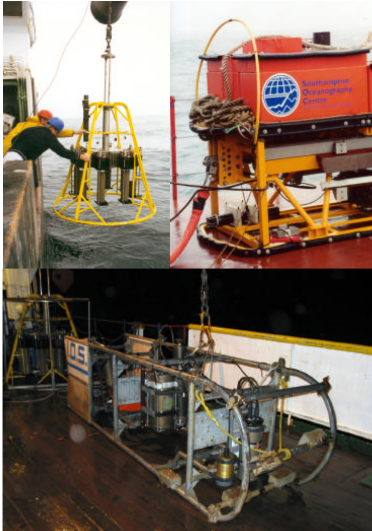
Seabed survey tools: top left – Megacorer; top right – TOBI sidescan sonar vehicle; bottom – WASP seabed photography system.
