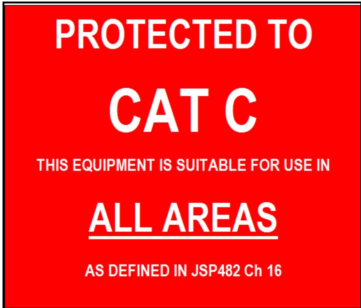
Figure 1: Signage to be affixed to MHE protected to enter all Category C environments (processing and storage etc.)
