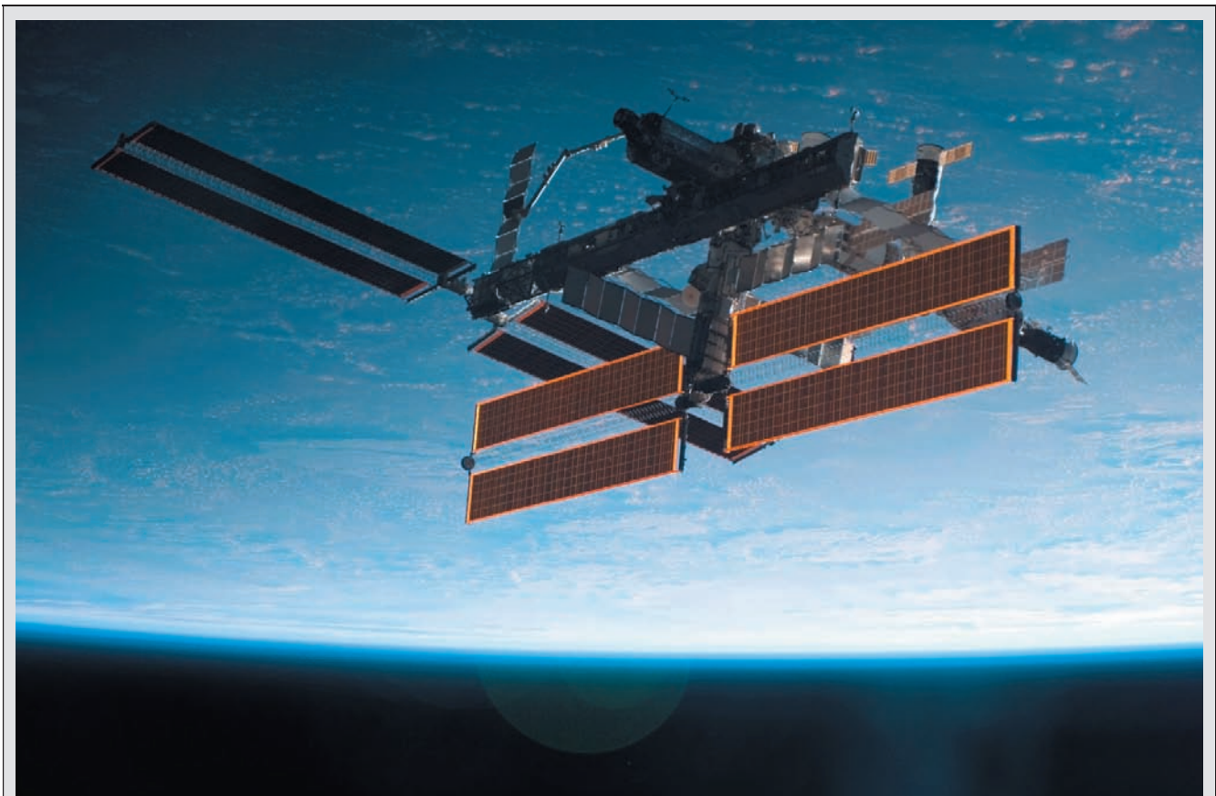
Illustration 1.37 – Power Generation in Space. The International Space Station (ISS) depends entirely on solar panels to generate electrical power. The extensive array of panels (at least 14 are visible in this image) is one reason that the ISS is so bright when seen in the night sky. Two Soyuz spacecraft are docked with the ISS in this view (top right corner and extreme right as seen here), each of which also has its own solar panel array extended. (NASA Image)
