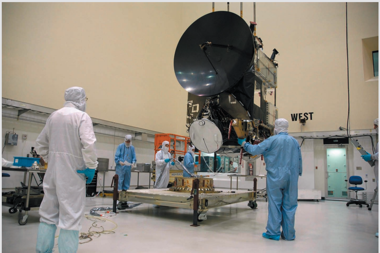
Illustration 1.6 – Mitigating Onboard Debris and Contamination. Engineers assemble a spacecraft (in this case NASA’s Dawn Interplanetary Probe) in clean conditions to avoid inclusion of any contamination or debris that might migrate in weightless conditions to an undesirable location. In this picture, the craft has yet to be covered in its thermal blanket. (NASA/courtesy of nasaimages.org).
