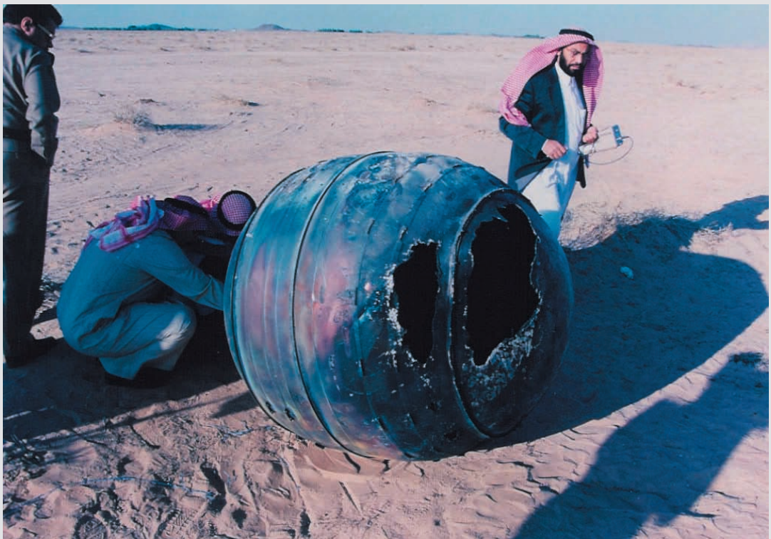
Illustration 1.34 – Uncontrolled Re-entry. The dangers of uncontrolled re-entry of spacecraft components are illustrated here in a photograph of a Delta 2 third-stage motor casing which re-entered the atmosphere in 2001. Weighing about 70kgs, the titanium casing ended up in the desert about 240 km from Riyadh, Saudi Arabia. The attractions of intentional re-entry into a safe area (typically over-water) are apparent. (NASA Image)
