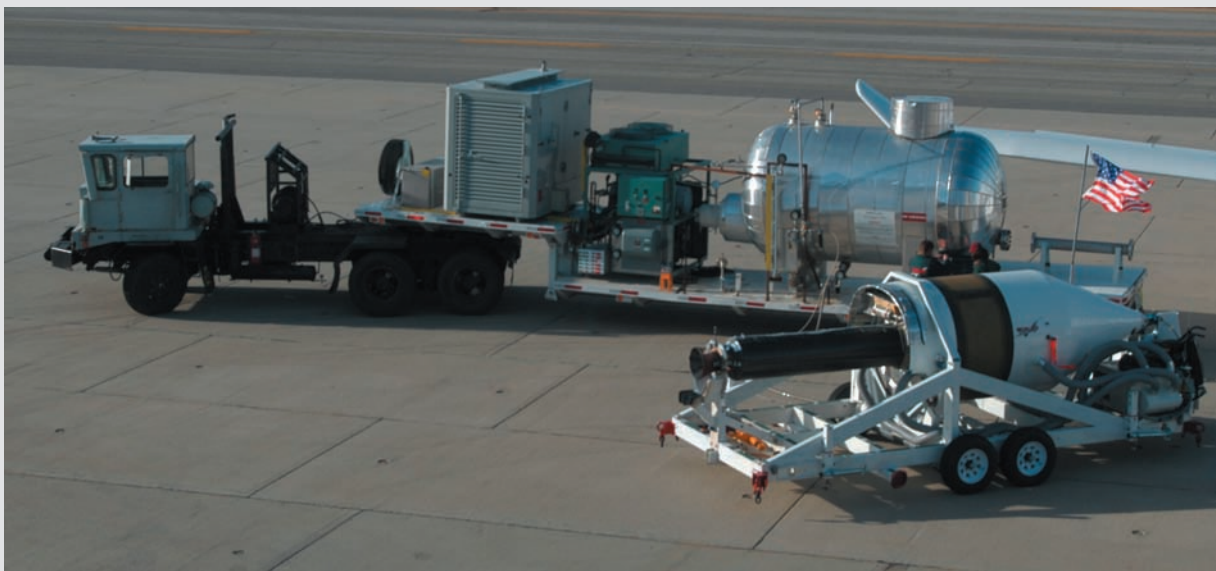
Illustration 1.27 – Hybrid Rocket Propulsion. This picture shows (foreground) the hybrid rocket motor used in SpaceShipOne built by Scaled Composites LLC in Mojave, California which won the Ansari X prize for private space-flight in 2004. The motor is mounted here in its test stand; the solid fuel is the cylinder and nozzle protruding at the rear. The large metal tank in the background is the ground storage and delivery system for the oxidizer (nitrous oxide in this application). As fitted to SpaceShipOne, the engine is not designed to provide thrust control (i.e. a throttle) to the pilot. It is, however, intended to support shut-down and re-start during a flight. (Image © 2004 Mojave Aerospace Ventures, LLC. SpaceShipOne®, A Paul G. Allen Project).
