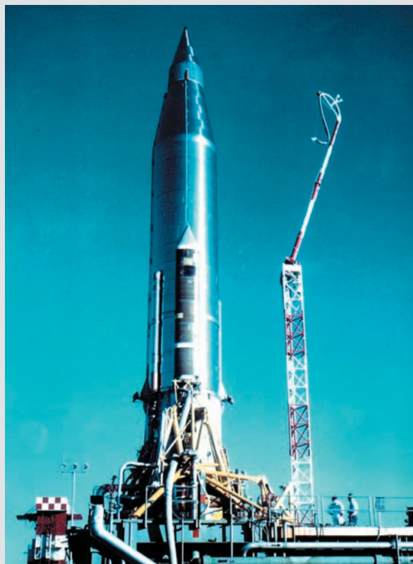
Illustration 3.5a – The Project SCORE Launcher. Seen just before launch, the SCORE payload mounted on an Atlas booster. (Picture courtesy of USAF)
