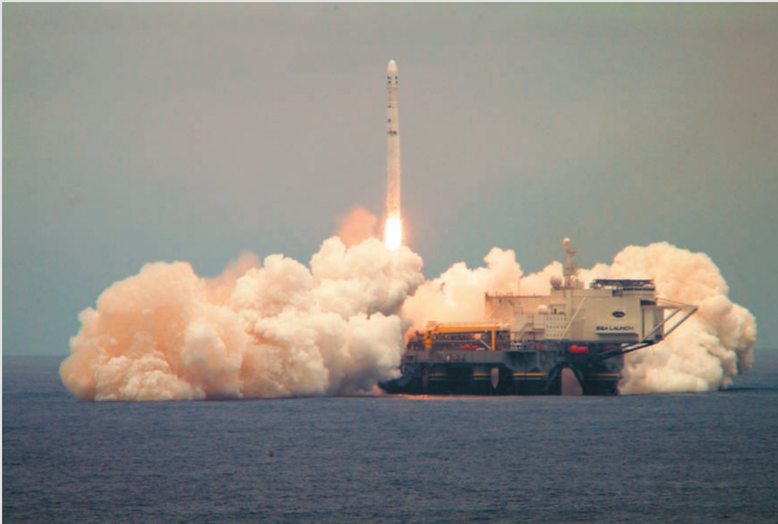
Illustration 1.29 – Sea Launch. The Sea Launch Company’s Odyssey launch platform illustrates one advantage of sea-launch. This launch is of the DirecTV11 broadcast satellite, using a Zenit-3L launcher to place a Boeing-built commercial broadcast satellite in geo-stationary orbit. The launch took place from the equator to maximise the contribution to launch velocity made by the Earth’s rotation. (Image courtesy of SLC)
