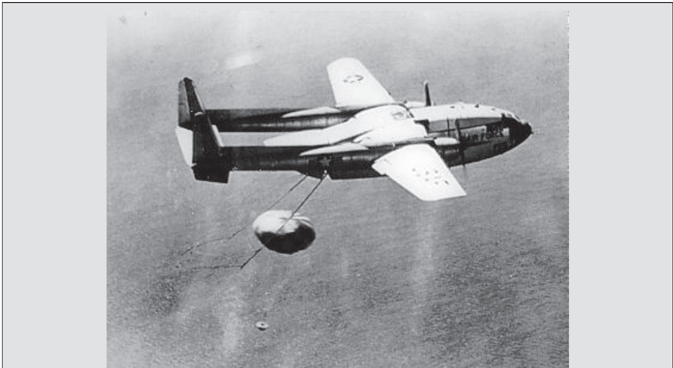
Illustration 1.35 – Returning Small Payloads. This picture shows a USAF C-119 transport aircraft capturing a film capsule returned from Earth orbit by an early reconnaissance satellite. After the ‘trapeze’ mechanism snagged the parachute, the capsule was winched back into the aircraft via the ramp and the undeveloped film retrieved for processing. C-130 aircraft were also used for the purpose. Despite its unwieldy appearance, the system proved rapid and reliable enough for regular employment between 1960 and 1972, although a similar system had a very public failure in 2004, when the NASA Genesis mission, due to return particles sampled from the solar wind to Earth, suffered a parachute failure and eluded the helicopters waiting to capture it near Salt Lake City, Utah. (USAF Picture)
