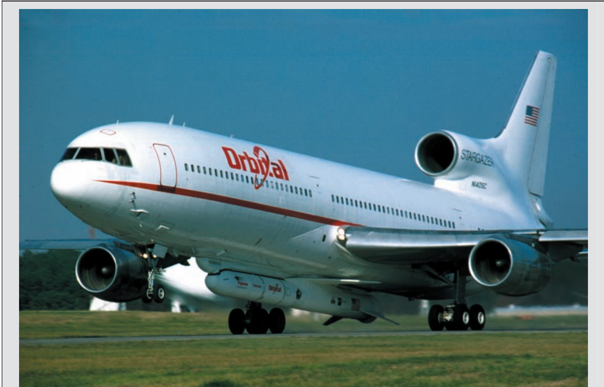
Illustration 1.30 – Air Launch. Orbital Science Corporation's (OSC) 'Stargazer' converted L1011 TriStar takes-off, carrying a 'Pegasus' launch vehicle capable of placing satellites in LEO. The pace of Pegasus launch activity has reduced in recent years as OSC have developed other conventional launchers, but the Stargazer/Pegasus combination proved the concept of commercial air-launch. (Image courtesy of Orbital Sciences Corporation). See also Illustration 4.3 in Chapter 4.
