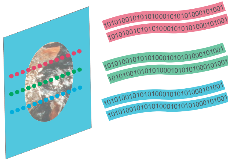
Illustration 3.16b – Multi-spectral Imaging 2. Each filtered array is read out repeatedly, and reassembled to give red-filtered, blue-filtered and green-filtered views of the target scene. These can then be combined to yield a colour (multi-spectral) image. For specific systems, the colours chosen for filters may vary (they may, for example include an IR sensing array), there may be more than 3 of them (though there will be a physical limit on how many can be fitted onto the focal plane), and their layout may be more complex than shown, but we have captured the principles of such a system.
