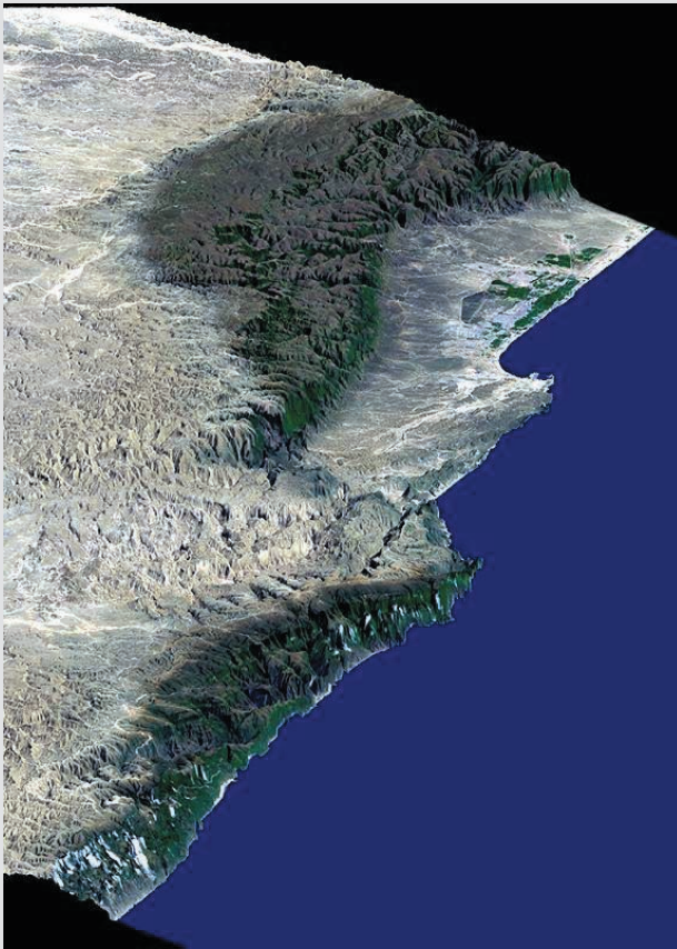
Illustration 4.1 – Earth Resources Monitoring. This image was derived from a combination of 2 space-derived datasets, gathered in 1999 and 2000. The terrain model showing the relief features came from the Space Shuttle Radar Topography mission, which generated a 3-D Earth model using radar measurements (actually the same transmitter as was used for the illustrative SAR image in Illustration 3.17, though on a different mission). The colour data was then supplied by the NASA Landsat satellite, which was overlaid on the terrain model. The terrain perspective was deliberately exaggerated by a factor of 3 in this image for clarity, which was used to track habitation, cultivation and the limits of desert. The target area is Salalah and the surrounding mountains and coastline in Oman. (NASA JPL Image)
