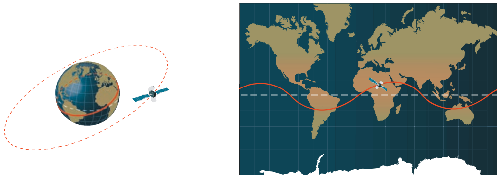
Illustration 1.18b – Ground Track for a Circular, Inclined Orbit. The satellite illustrated above is in a circular, inclined orbit. It will spend half its time over the northern hemisphere, and half over the southern hemisphere (a consequence of the plane of the orbit passing through the centre of the Earth, in accordance with Kepler’s First Law). The inclination of the orbit (see Illustration 1.17) limits the latitude of the points it can overfly. In the example shown, the satellite orbit is inclined at 20^\circ to the Equatorial Plane, and the ground track is restricted to lie between latitudes 20^\circ\text{N} and 20^\circ\text{S} .
