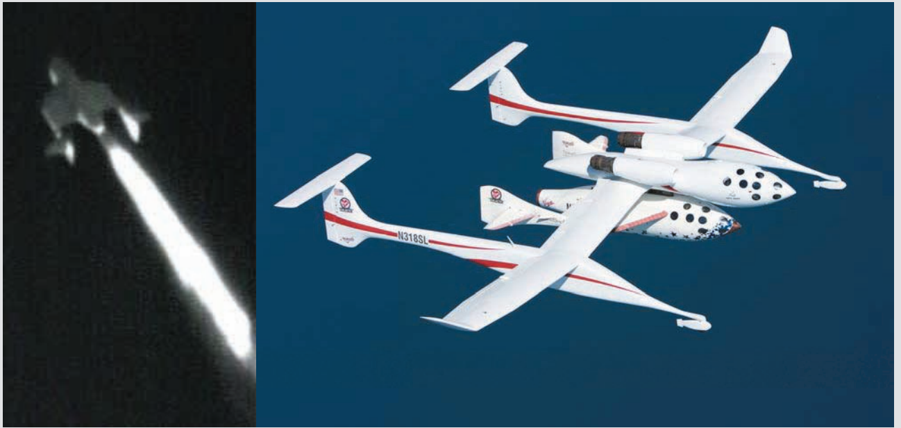
Illustration 4.3 – Space Tourism. The Virgin Galactic company intend to offer private space travel on a commercial basis. The images show (left) SpaceShipOne being carried aloft by the WhiteKnightOne launch platform and (right) SpaceShipOne in sub-orbital flight (travelling at about 2500 mph when this photo was taken). This combination won the Ansari-X prize for private spaceflight in October 2004, and forms the basis for development of the operational commercial vehicle. Other potential uses of such vehicles, such as scientific research and small satellite launch are being considered. (Image courtesy of Virgin Galactic LLC).
