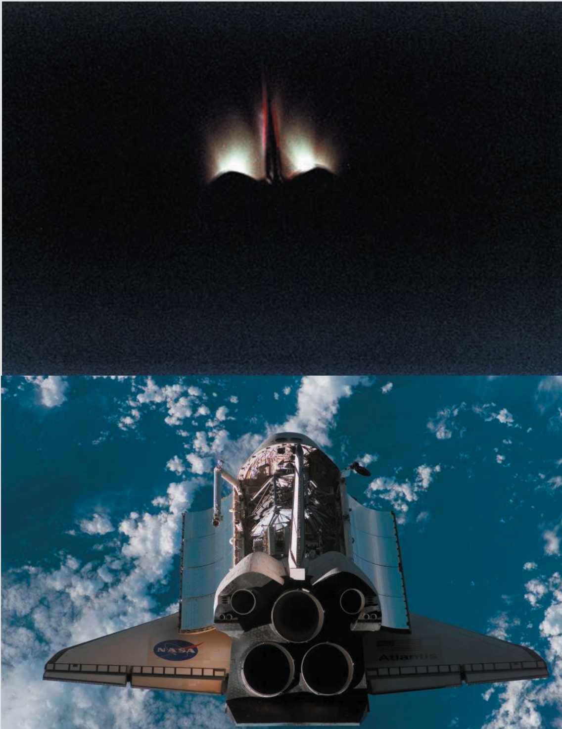
Illustration 1.31 – Orbital Manoeuvring. Orbital manoeuvres by satellites usually takes place out of sight of any human observers, but these photographs capture what happens. The top picture shows the instant of the Space Shuttle Atlantis firing its Orbital Manoeuvring System (OMS) engines during flight STS-84 in May 1997. The OMS engines are at the rear of the Shuttle, separate from the main engines, and use hypergolic fuel (see Paragraph 157a). They provide the final push into orbit on each Shuttle launch after the main engines shut down, and are also used to boost orbital altitude when coupled to the ISS. In the upper image, the exhaust highlights the vertical fin, as seen from the flight deck looking aft. The lower image shows a range of Space Shuttle engine exhausts: the Main Engines (3 largest exhausts), the OMS engines (two smaller adjacent exhausts) and the rear portion of the Reaction Control System for attitude control (small nozzles facing aft and upwards outboard of each OMS engine). The windows through which the upper image was taken can also be seen at the forward end of the payload bay. (NASA Shuttle-Mir History images)
