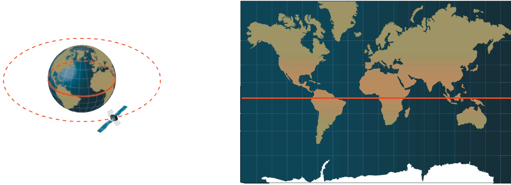
Illustration 1.18a – Ground Track for a Circular, Equatorial Orbit. The satellite above is in orbit over the equator. For a low-earth orbit, its period will probably be in the range 90-120 minutes (for clarity, the satellite in the illustration is drawn at a much greater altitude). Its path will lie above the equator, overtaking the Earth smoothly.
