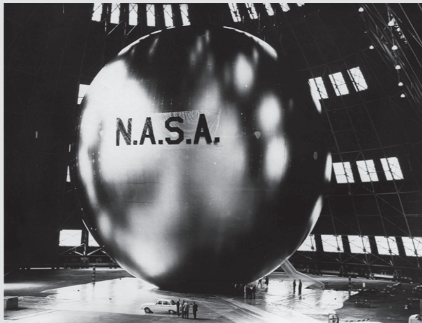
Illustration 3.4 – A Passive Communications Satellite. The picture shows a test inflation of the NASA ‘ECHO’ satellite in a hangar. The operational satellite was launched into orbit then inflated, where it acted as a passive reflector for ground transmissions. Note the onlookers and their saloon car to gain a sense of scale. The associated ground installation is illustrated in Chapter 1. Although the principle proved successful, active satellites quickly supplanted such systems. (Image courtesy of NASA).
