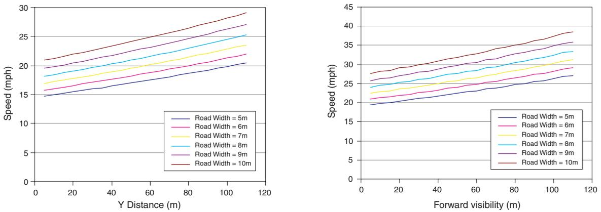
**Figure 5.5** Junction model – manual speeds with average site features (non-turners only)
