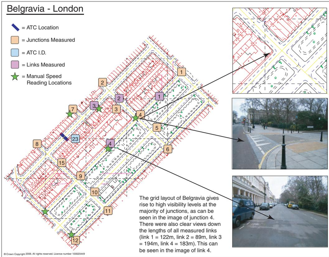
**Figure 4.5** Belgravia – grid layout (large visibilities)
