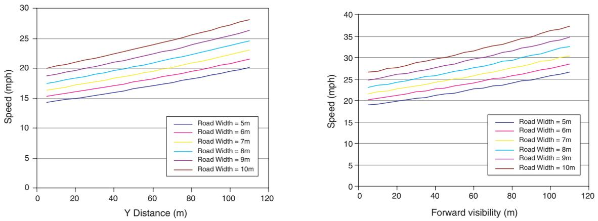
**Figure 5.4** Junction model – manual speeds with average site features (all vehicles)
