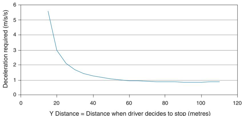
**Figure 6.4** Deceleration rate required by second vehicle to stop if seeing first vehicle at 'Y-distance' metres from junction
