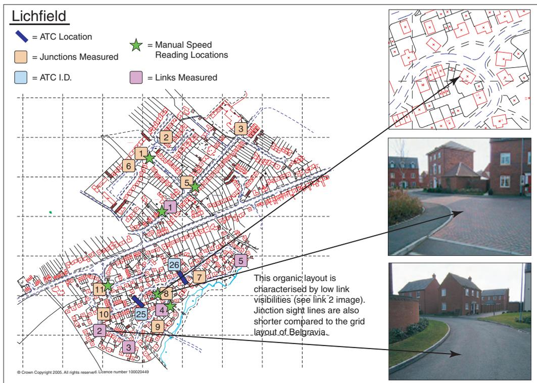
**Figure 4.4 Lichfield – non-grid layout (limited visibilities)**
