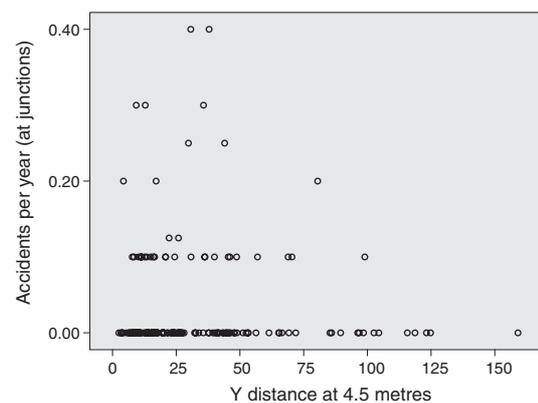
**Figure 7.4** Junction accidents – according to Y-distance
