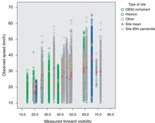
**Figure 4.6** Speed ATC data for links (by site type)
