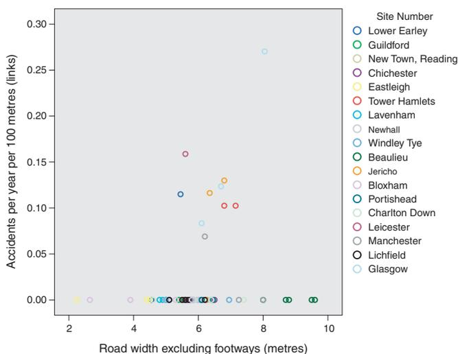
**Figure 7.8** Link accidents per 100 m – according to road width
