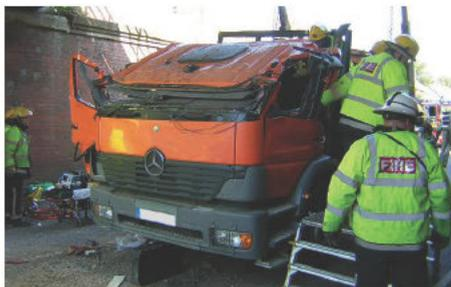
Crushed cab of a skip lorry following a bridge strike
