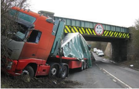
*Damaged vehicle and load following a bridge strike*
