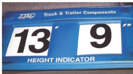
Notice in a driver's cab displaying the overall vehicle height
