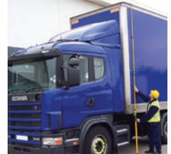
Checking the height of a trailer using a telescopic measuring device
