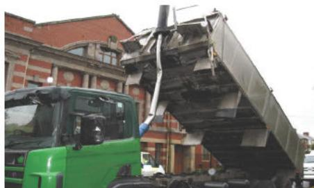
Result of tipper vehicle equipment not correctly loaded striking a bridge
