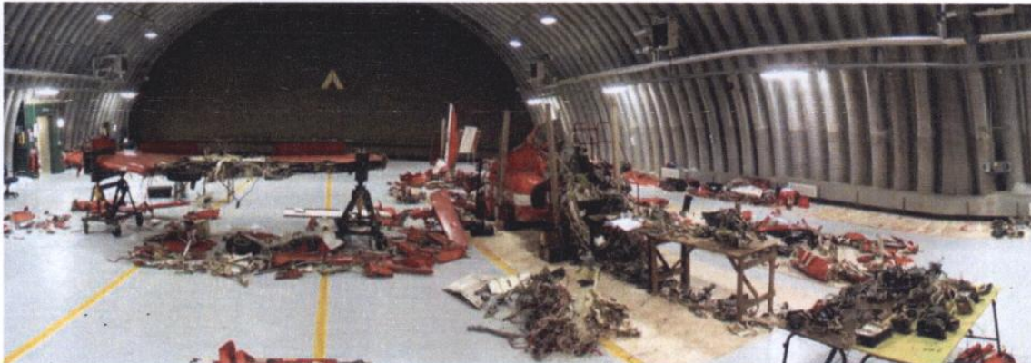
Figure 2 – XX179 lay out in MOD Boscombe Down as part of the engineering investigation.
