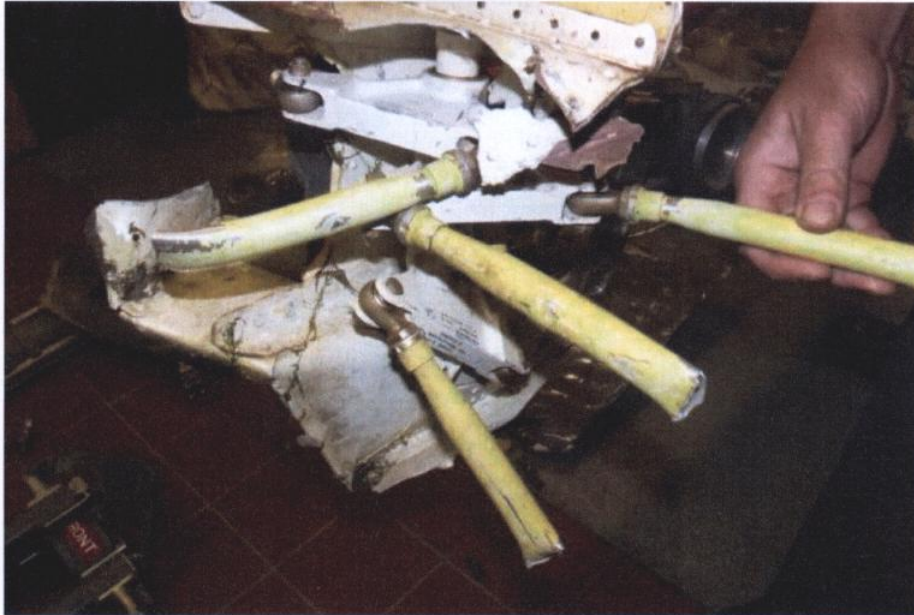
Figure 5 – Typical example of XX179's damaged control rods post accident.
