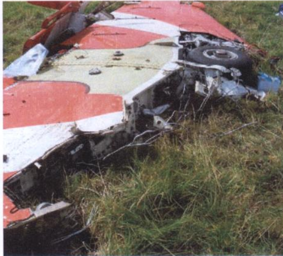
Figure 7 – Underside of wing with right hand main wheel in the retracted position.
