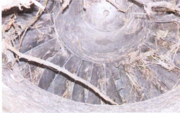
Figure 3 – The forward face of the compressor as viewed through the left hand air intake.
