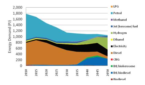
Figure 11: Energy Consumption in the Transport Sector in DECC-1A-IAB-2A
