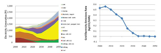
Figure 4: Emissions Intensity Reduction for Grid Electricity in Run DECC-1A-IAB-2A
