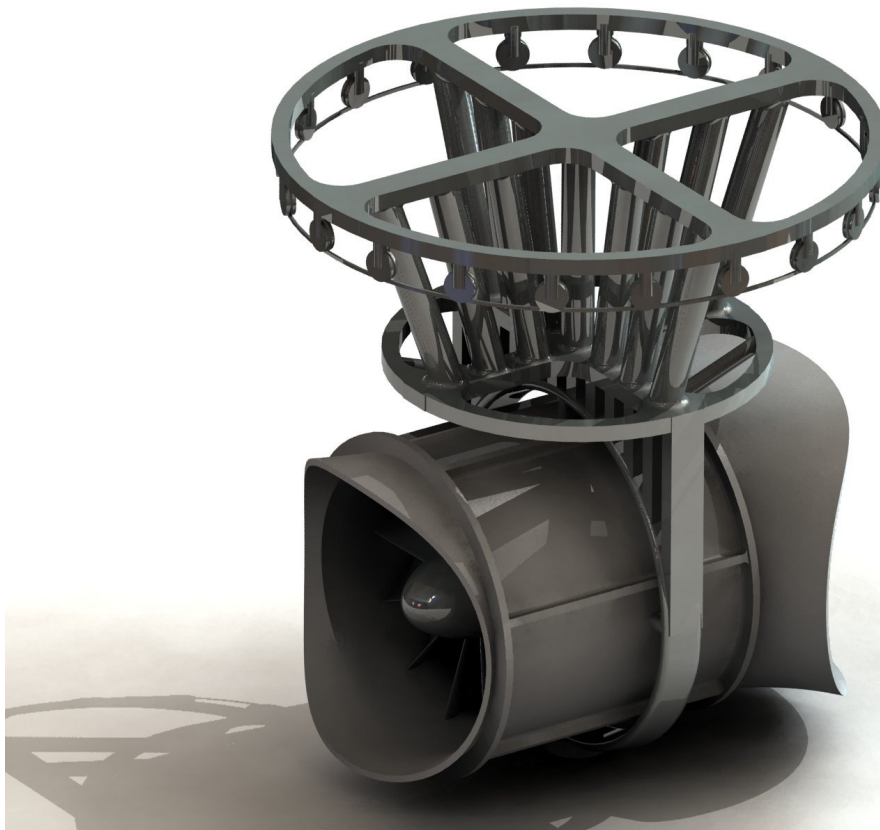
Figure 7 Red turbine configuration developed under SETS.
