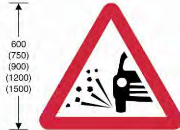
7009 Loose chippings on road ahead
