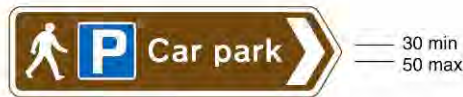
2609 Direction of route for pedestrians to a parking place associated with a tourist attraction
