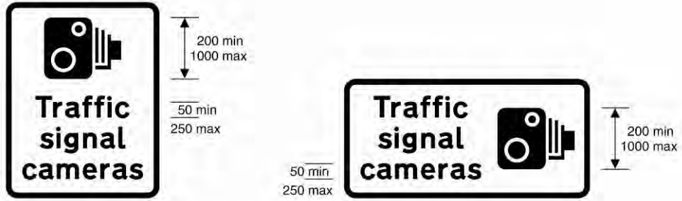
878 Area in which cameras are used to enforce traffic regulations (Alternative types)
