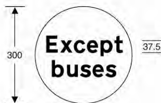
954.5 Same as diagram 954 where the signs are mounted in combination with light signals prescribed by regulation 33
