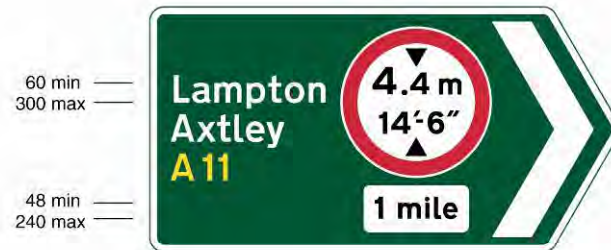
2027 Direction to a primary route along which there is a height restriction
