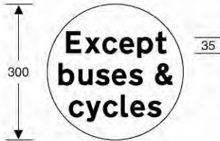
954.6 Same as diagram 954 applying to buses and pedal cycles where the signs are mounted in combination with light signals prescribed by regulation 33
