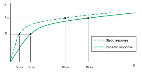
Figure 19: Static and dynamic responses derived from energy balance © Arup
