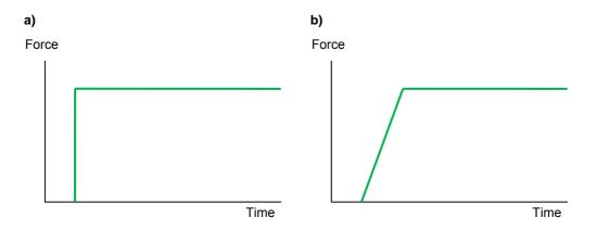
Figure 20: Application of gravitational load in a dynamic time history analysis a) Instantaneous column loss b) Sudden but non-instantaneous column loss
