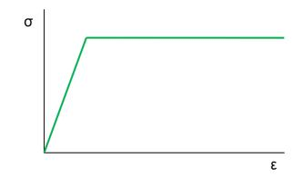
Figure 12: Linear elastic-perfectly plastic material model
