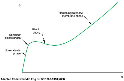
Figure 16: Phases of ultimate failure
