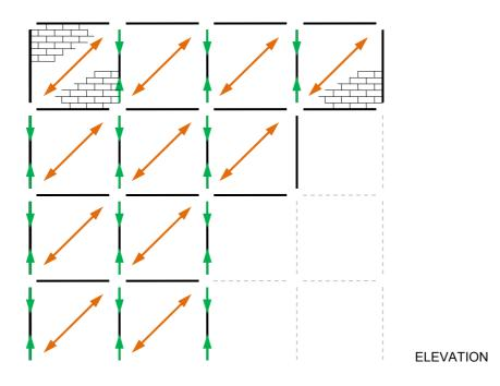
f: Mechanisms to resist collapse. Compressive strut action in masonry panels
