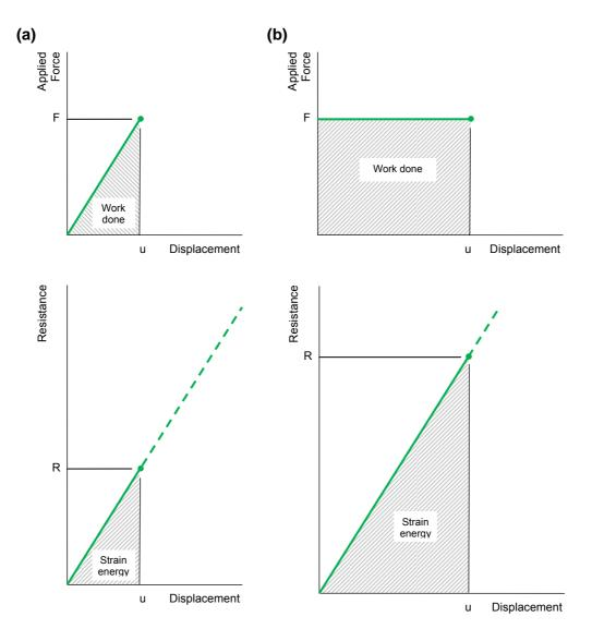
Figure 17: Work done versus internal energy in a linear elastic system a) static load b) suddenly applied dynamic load © Arup
