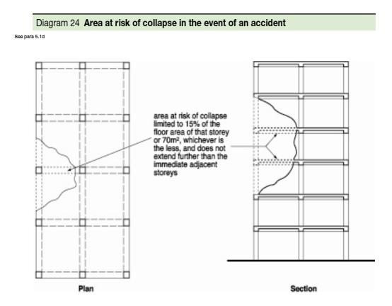
Ref: The Building Regulations 2000 – Approved Document A: 2004: Structure – A3: Disproportionate Collapse Figure 3: Approved Document A: 2004 Diagram 24: Area at risk of collapse in the event of an accident
