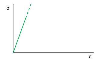
Figure 11: Linear elastic material model
