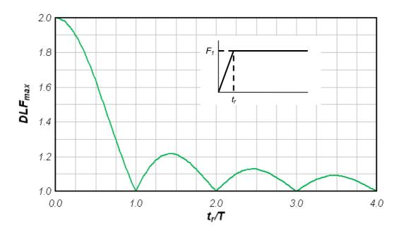
Figure 15: Maximum response of one-degree elastic systems (undamped) subjected to constant force with finite rise time (US Army Corps of Engineers: Design of structures to resist the effects of atomic weapons. Manual EM 1110-345-415, 1957).
