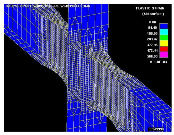
Figure 22: Moment-resisting seismic connection with reduced flange widths. © Arup
