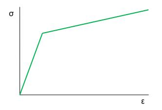
Figure 13: Linear elastic-plastic material model with strain hardening
