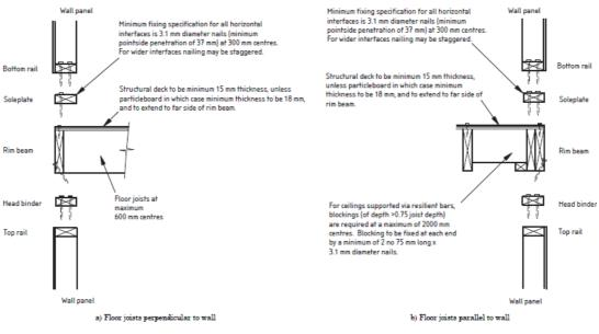
${\rm Figure}\;{\rm M.3-Floor\;deck-wall\;panels\;intersection}; {\rm Exploded\;view}$
