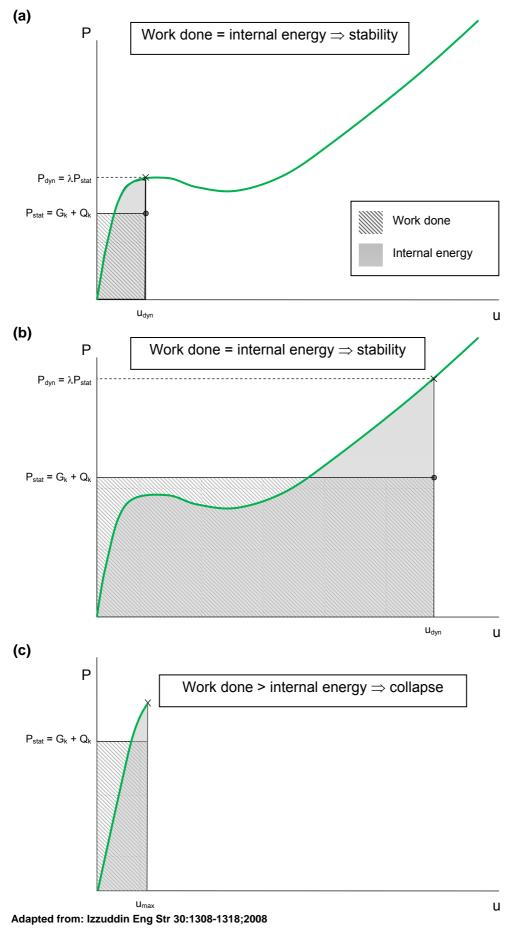
Figure 18: Work done versus internal energy for real structural systems © Arup
