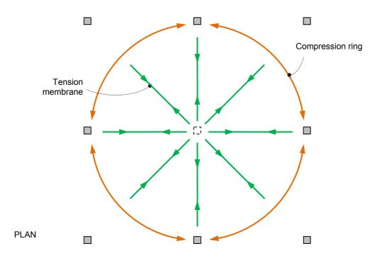
c: Mechanisms to resist collapse. Tensile membrane developed in a flat slab after the removal of the central column.
