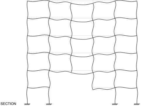
d: Mechanisms to resist collapse. Vierendeel action due to moment capacity in beam/column connections following loss of two columns (of which one is lost over two storeys) and the first floor beam over two structural bays.
