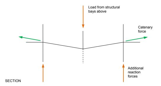
Figure 10: Mechanisms to resist collapse a: Mechanisms to resist collapse. Catenary action in structural beam/column frame of an internal column after removal of a supporting column.
