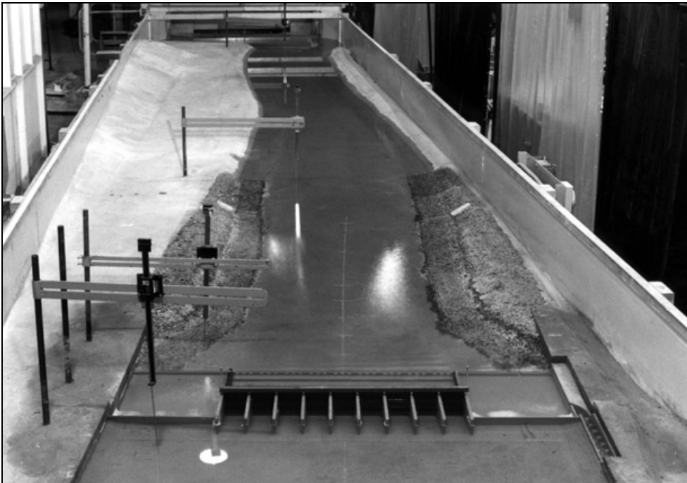
Fig. 5. Photo of plan model viewed from upstream
