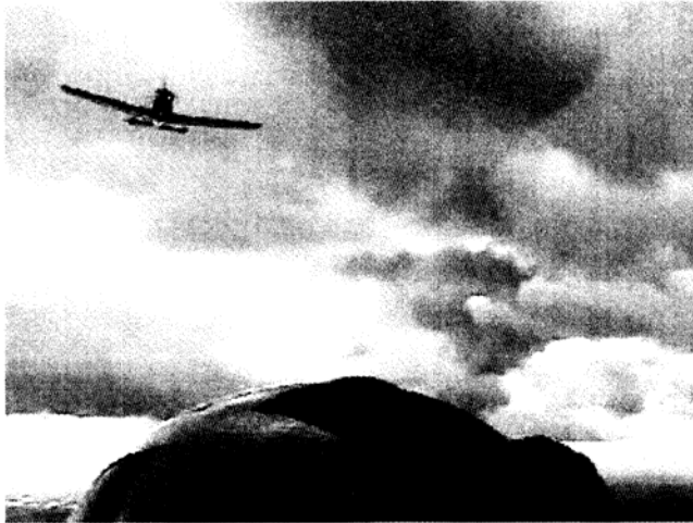
Figure 26. Reconstruction flight: estimated view from G-BYVN of Tutor simulating G-BYUT approximately 1 sec prior to the simulated collision point. Note the elevated camera to achieve an unobstructed view over the adjacent seat occupant. In the reconstruction, height separation was maintained.
