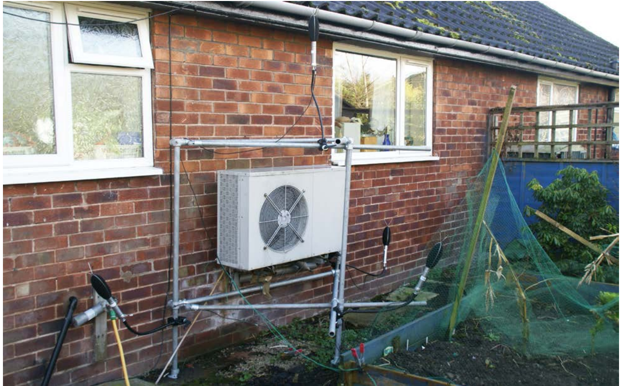
Picture 5-15. 443 Cheshire West, ASHP and Microphone Arrangement
