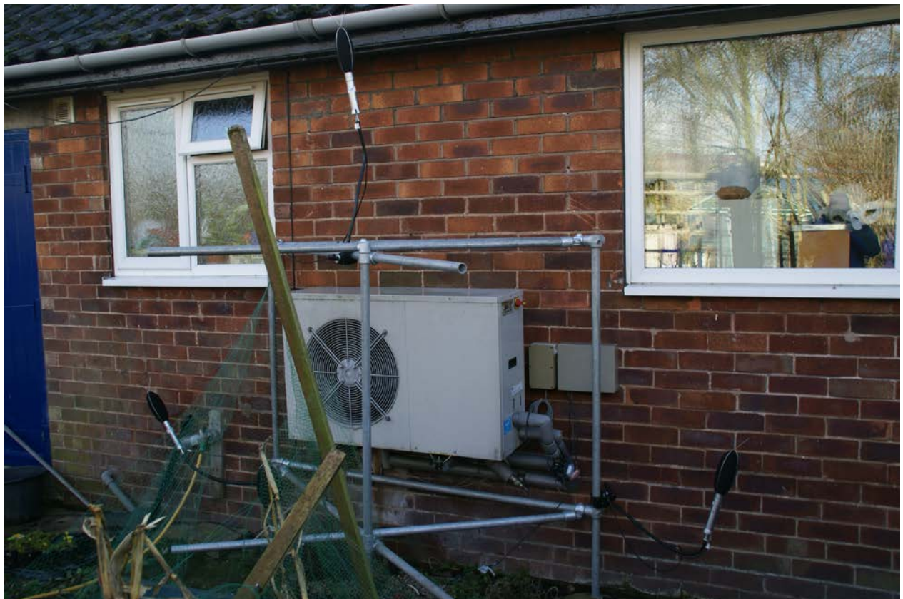
Picture 5-16. 443 Cheshire West, ASHP and Microphone Arrangement
