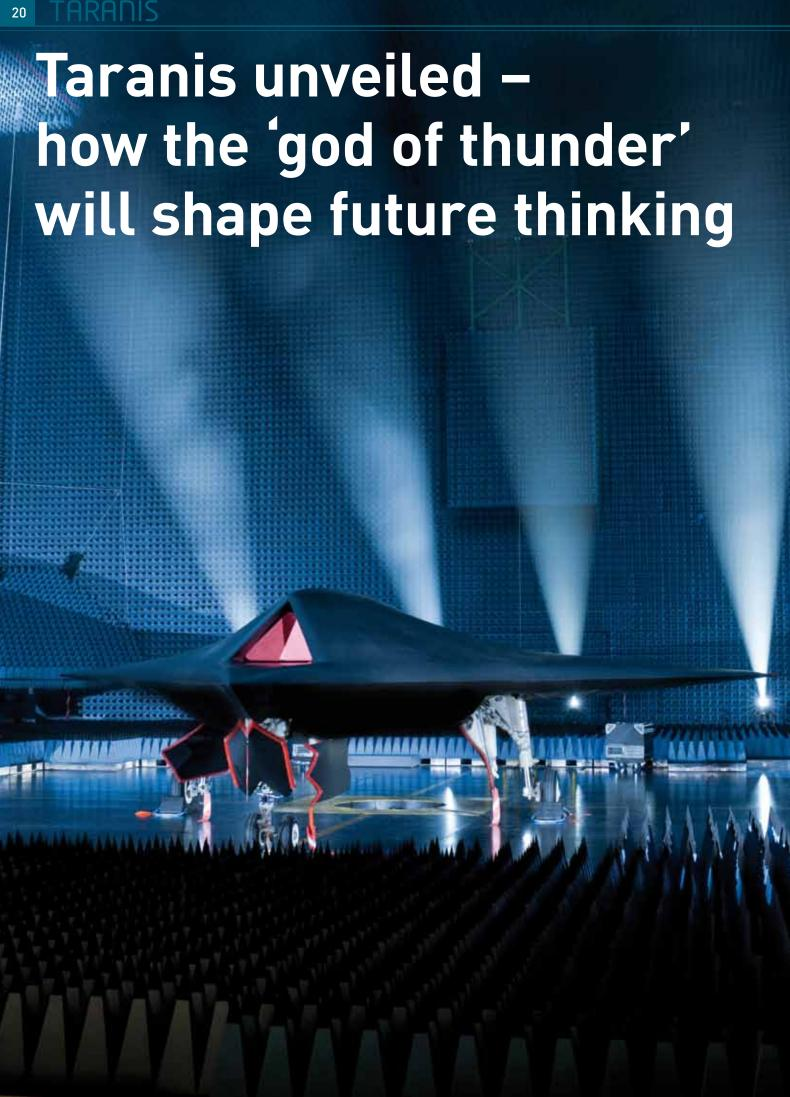
n unmanned combat aircraft of the future - Taranis - has been unveiled. Named after the Celtic god of thunder, the 12m long concept demonstrator with a wing span of 10m will test the possibility of developing the first ever autonomous stealthy Unmanned Combat Air Vehicle which would ultimately be capable of precisely striking targets at long range, even in another continent.
