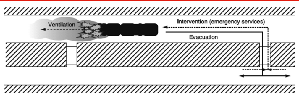
Picture 3: Standard procedure for dealing with an incident in a twin bore tunnel via the unaffected bore and crossovers
