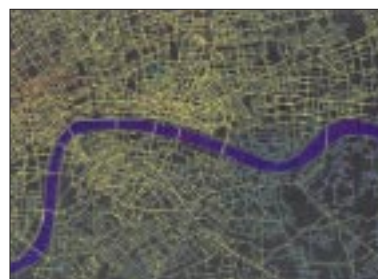
▲ SPACE SYNTAX IS A TECHNIQUE FOR MEASURING HOW WELL STREETS ARE CONNECTED
