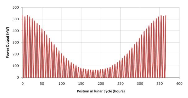
**Figure 9:** Power output from an MCT (Deep – 14m diameter rotor) type TEC device over one lunar cycle (spring to spring – 366 hours approximately
