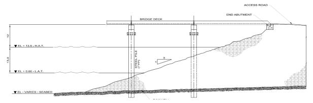
Figure 14: Drawing showing an example landfall causeway at the end of the fence.
