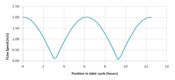
Figure 6: Flow speed over one tidal cycle (12.4 hours approximately) during peak spring tides
