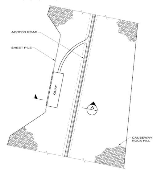
*Figure 15:* Drawing showing an example quay built into the side of the landfall causeways. These quays (at either end of the fence) will serve maintenance vessels required when the access bridge is insufficient.
