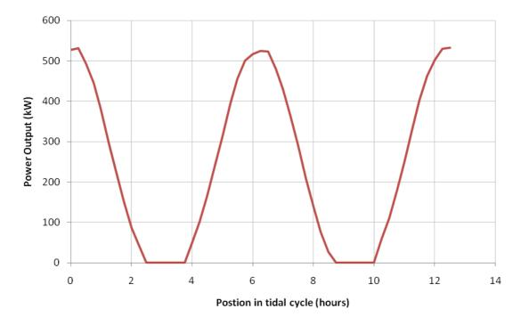
*Figure 7:* Power output from an MCT (Deep – 14m diameter rotor) type TEC device over one tidal cycle during peak spring tides
