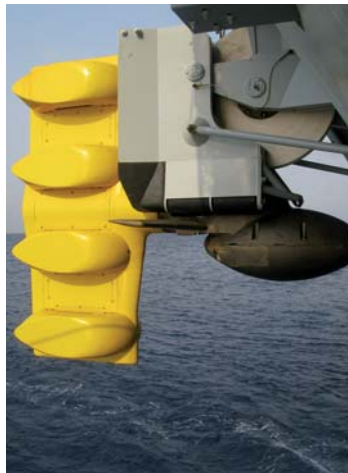
Above: the body for the towed array of Sonar 2087 on HMS Sutherland
