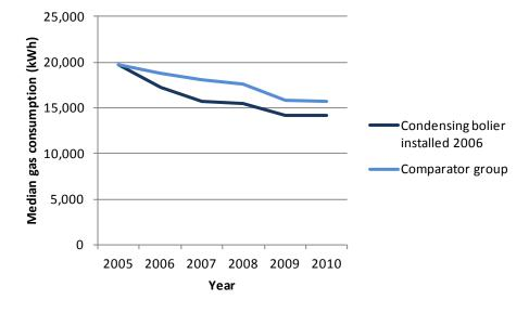
Figure 5.4: Condensing boiler installed in 2006 – long term gas consumption
