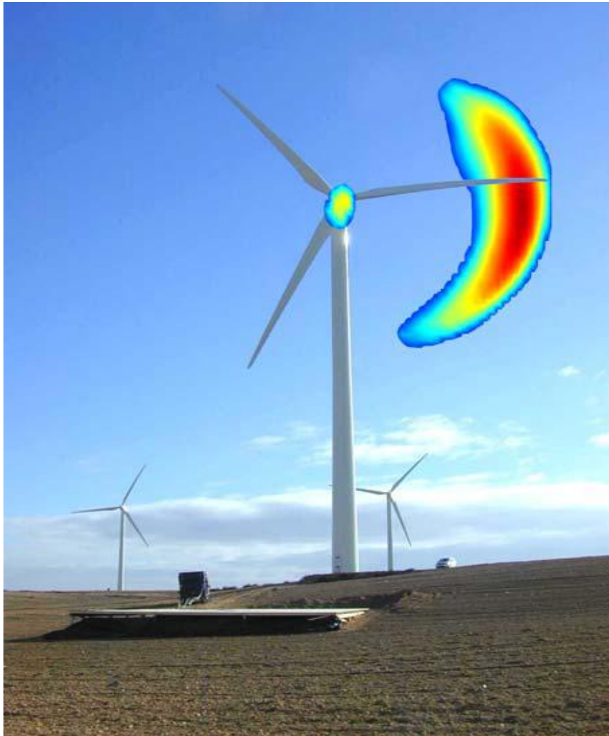
Figure 3 Test set-up with G58 turbine and microphone array platform. The noise sources in the rotor plane (averaged over several rotations) are projected on the picture - Oerlemans S, Lopez BM, Localisation and quantification of noise sources on a wind turbine, Wind Turbine Noise: Perspectives for Control Berlin 17th and 18th October 2005
