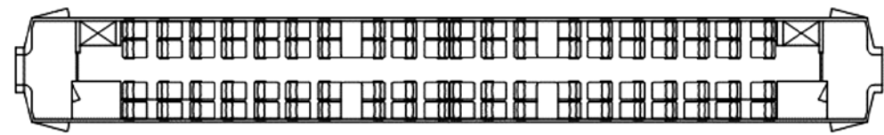
Plan – luggage stack and toilet each end, internal sliding door between vestibule and saloon
