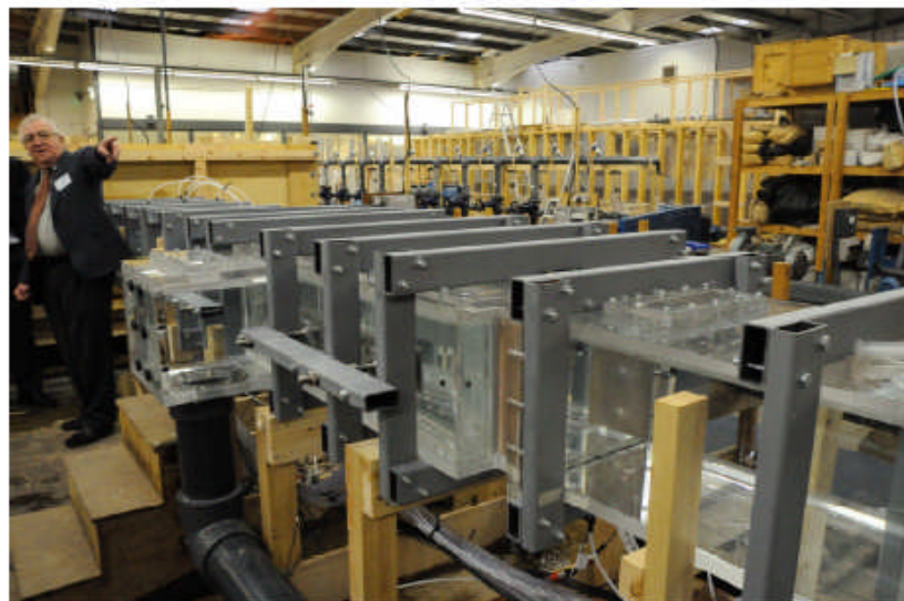
Test Section in foreground feeding into the Modular Receiving Tank
