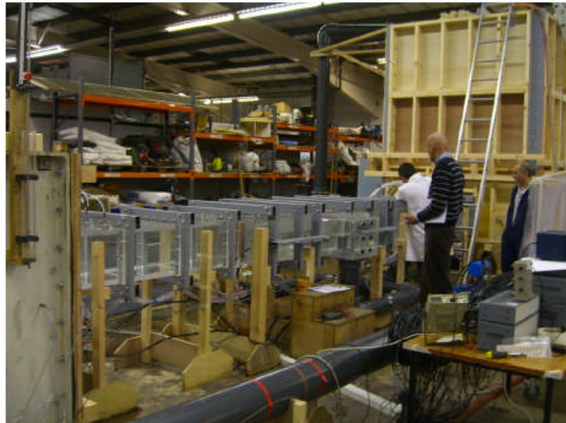
Upstream Feeder Tank to right, Modular Receiving Tank to left
