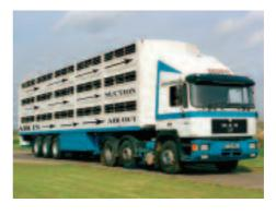
(headboard) end. So, with a vehicle moving at speed, air will enter the container through the rear vents, move forward over the animals, and leave through the front vents.
