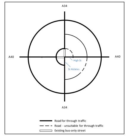
Figure 2.6 - Schematic of Oxford road network showing the function of High St and St Aldates
