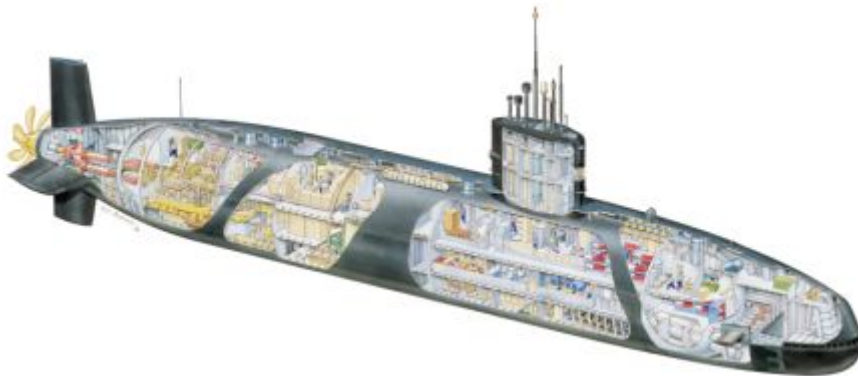
Figure 1 - Cross-Section of a Royal Navy 'T' Class Submarine, showing the location of the Reactor Compartment. (Crown Copyright - Navy News).
