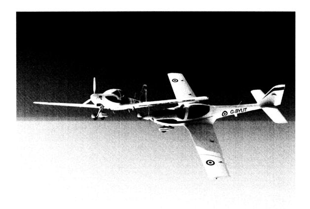
Figure 4. Collision orientation: nose of G-BYUT impacting port main wheel of G-BYVN.
