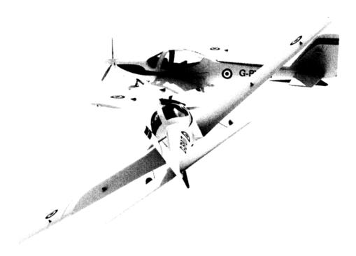
Figure 3. Collision orientation: starboard wing of G-BYUT impacting rear fuselage of G-BYVN.
