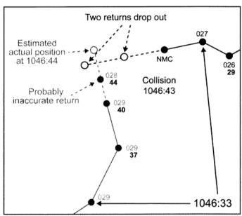
Figure 8. Assessment of returns affected by radar resolution cell.
