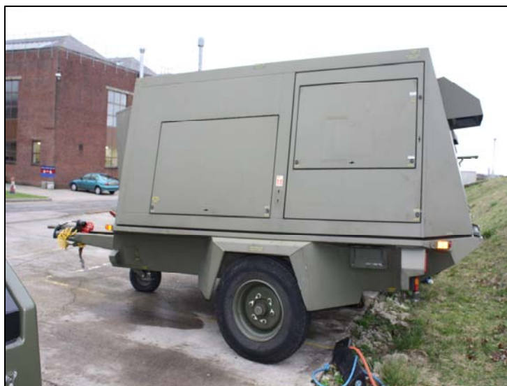
Figure 7.2 – Field Electrical Power System
