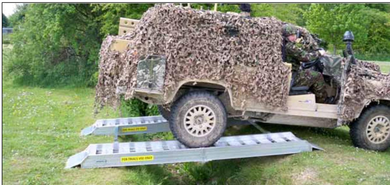
Figure 2.4 – Short gap crossing equipment
