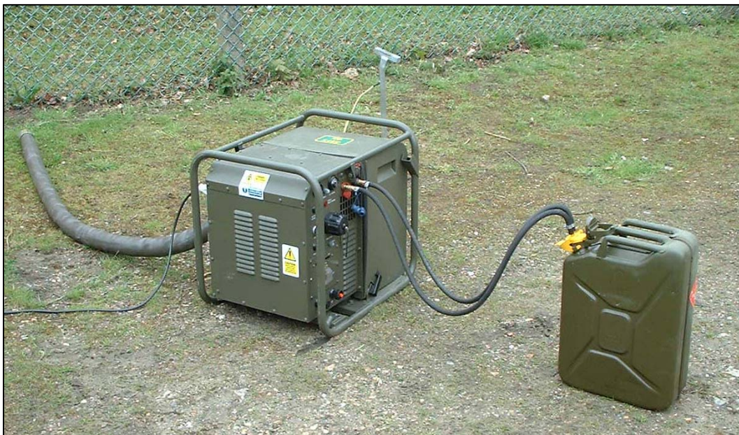
Figure 7.1 – Lightweight Field Generator
