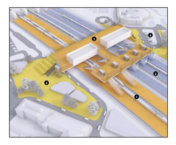
(3.2.12) The concourse bridge linking the two sides of the station would improve on the situation at the existing Derby station, where the current public pedestrian routes across the railway are limited to the underpass at the north end.
