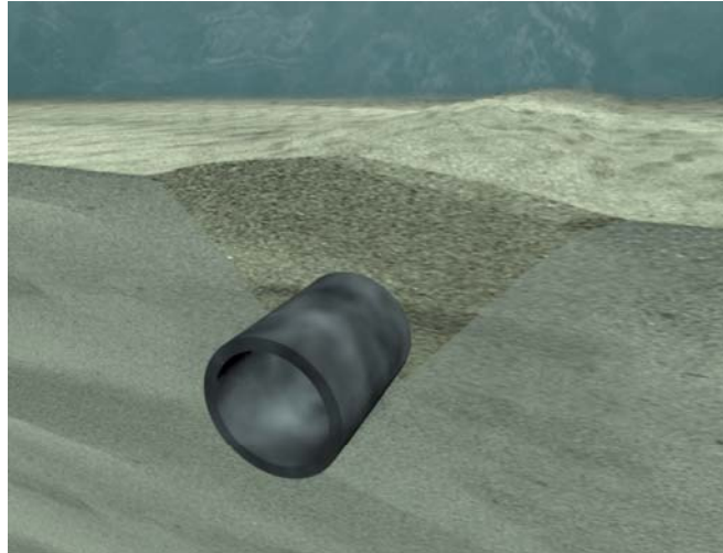
Figure 10.1: Trench and bury technique.
