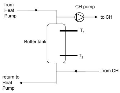
Figure 4.1: Buffer tank set-up
