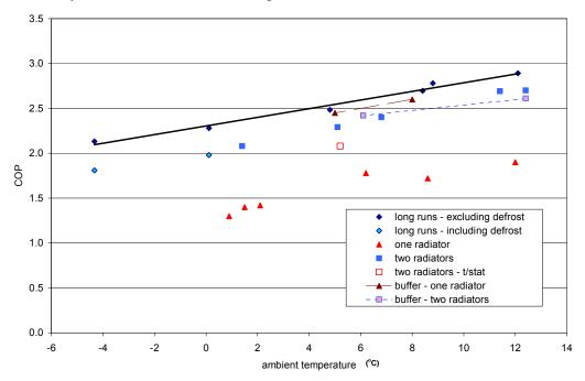
Figure 6.1: Comparison of forced cycling buffer results, with and without buffer tank
