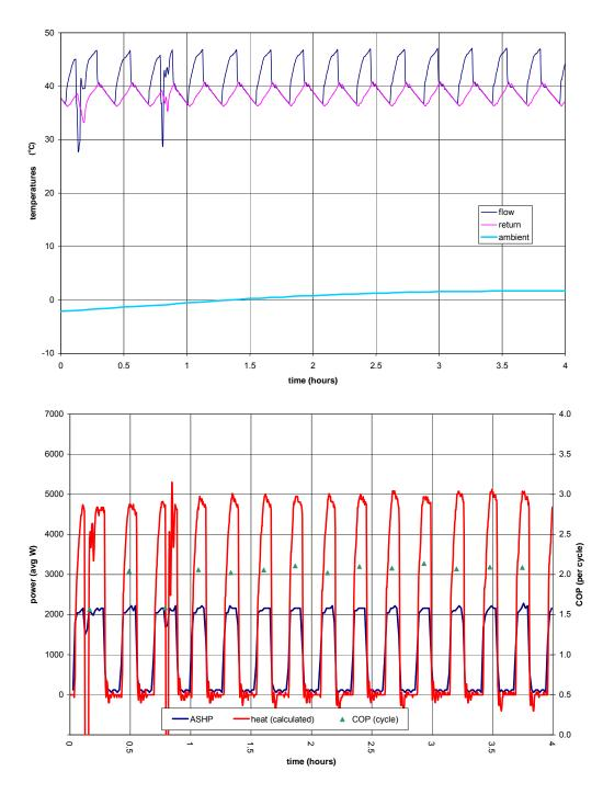
Run time:7.1 minutes(4 cycles in 64 minutes)COP:2.1 (~1.6 when cycle includes defrost –  $1^{st}$  and  $3^{rd}$  cycles in graphs)
