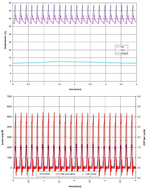
Figure 2.1: Example power & COP graphs (forced cycling, 1 radiator open)
