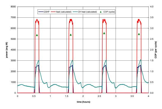
Figure 5.1: Power (heat and electricity) and COP (forced cycling, 1 radiator)
