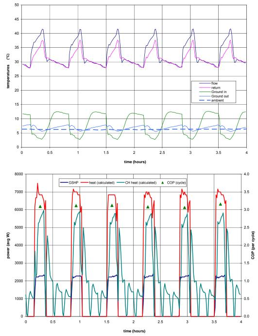
The lower graph shows the heat pump cycling regularly (blue and red lines). The Central Heating (the green line) cycles on and off during the heat pump off periods. This is due to the room thermostat being satisfied, and then calling for more heat.
