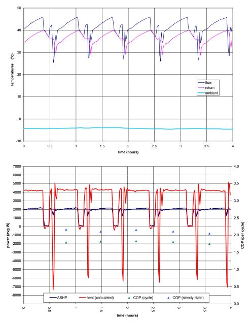
The "steady-state" COP is calculated for a 10 minute period towards the end of each run. The COP value for the complete cycle includes the defrost energy used.
