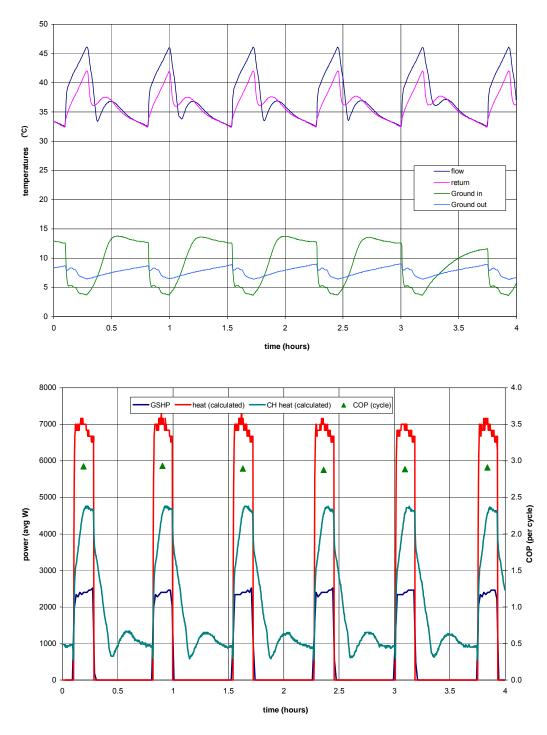
Average run time:10.7 minutesCycle time ~ 44 minutesmax  $T_{flow} = 46^{\circ}C$ Average COP:2.90 / 3.08average CH output ~ 1,800 W
