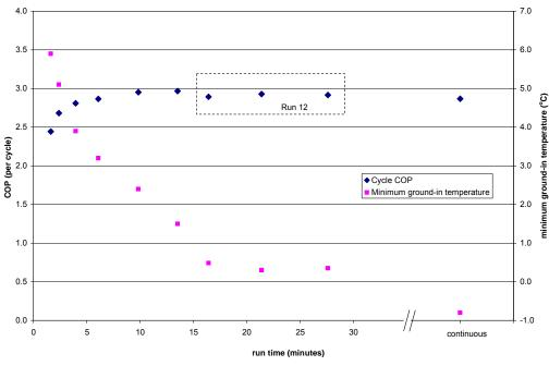
Figure 3.5: Summary of results including ground-in temperatures
