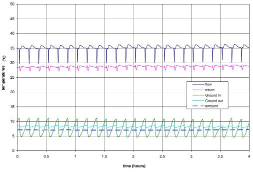
Figure 3.7: Full system operation under room thermostat control
