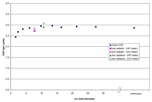
Figure 5.2: Comparison of GSHP forced cycling results with and without buffer tank
