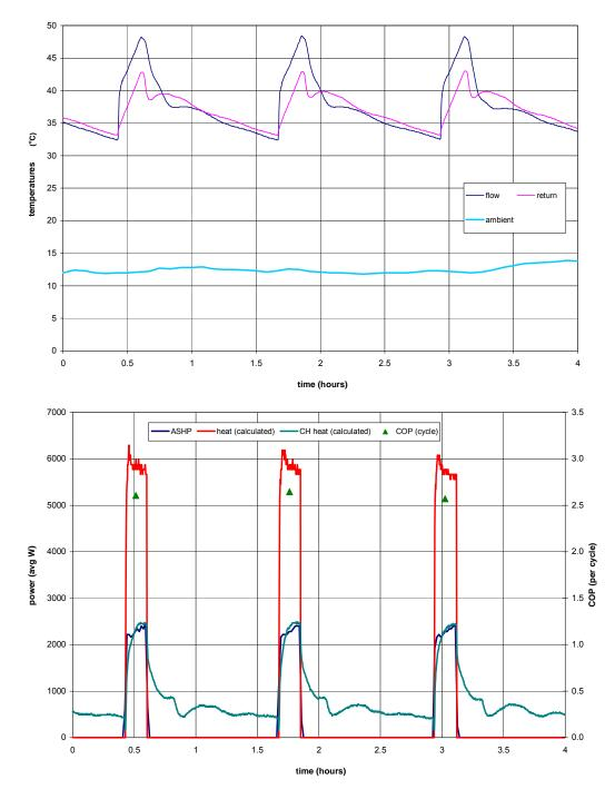
Average run time:10.8 minutesCycle time ~ 75 minutesmax  $T_{flow}$  = 48.1°CAverage COP:2.61average CH output ~ 730 W
