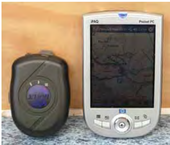
Figure 51: a PDA with map viewing software and GPS linked by Bluetooth wireless communications
