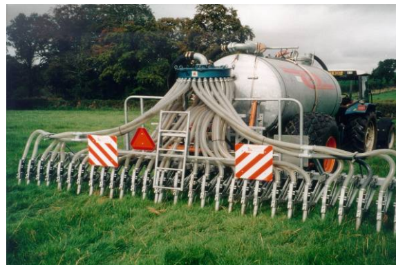
Plate 3. Trailing hose slurry application to winter wheat (left) and trailing shoe slurry application on grassland (right)
