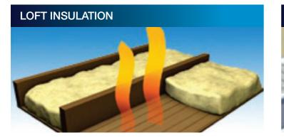
Loft insulation acts as a blanket, trapping heat rising from the house below. For optimum efficiency, pipes can be insulated at the same time. Some properties already have some loft insulation but you could increase this level to the optimal 30cm/12inches to further reduce your energy bills. Your existing loft insulation may also have deteriorated over the years.
