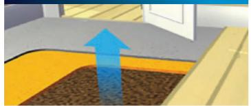
To retain heat and stop draughts, timber floors can be insulated by lifting the floorboards and laying mineral wool insulation supported by netting between the joists. You can also use a tube sealant, such as silicon, to fill gaps between floorboards and skirting boards.
