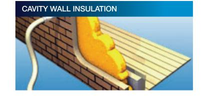
In most houses built after 1930, the external walls are made of two layers with a small air gap or 'cavity' between them; this results in a considerable amount of heat being lost. Cavity wall insulation fills the gap with an insulating material, which reduces the amount of heat that escapes through the walls and helps prevent condensation.
