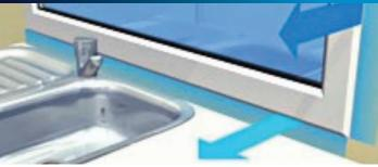
Draught-proofing means blocking up unwanted gaps that let cold air in and warm air out. The most common places where gaps lead outside are: windows; doors; loft hatches; electrical fittings on walls and ceilings; suspended floorboards; pipework leading outside; and ceiling-to-wall joints.
