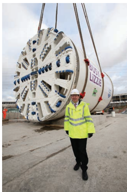
Figure 1: 'Busy Lizzie' Tunnel boring machine and Martin Baggs, Thames Water Chief Executive Officer
