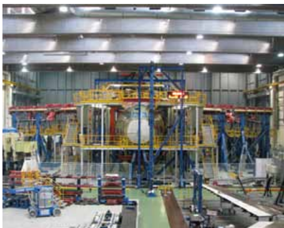
A400M wings have passed their ultimate bend test.
