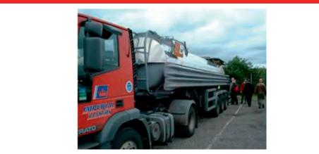
**7C3.200** The photo above shows a non-pressure tank containing Nitric Acid>70 per cent. Note the added protection to prevent accidental damage to the structure of the tank, which is a good indication that the tanker carries a high consequence load.
