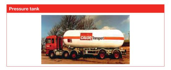
**7C3.203** The above photo shows a typical pressure tank designed for carrying liquid petroleum gas.
