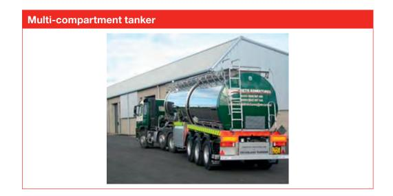
**7C3.201** The photo above shows a 30,000 litre non-pressure, stainless steel, multicompartment tanker that can carry a variety of substances at different times but only compatible loads during any single journey.
