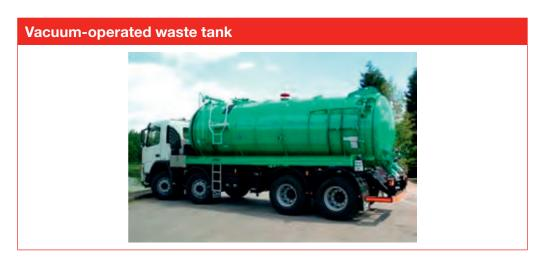
**7C3.202** The photo above shows a vacuum-operated tank; notice should be taken of the external strengthening ribs which are to prevent the tank collapsing when the vacuum is applied. Details of the specifications regarding vacuum operated waste tanks can be found in Chapter 6.10 of ADR Volume II.
