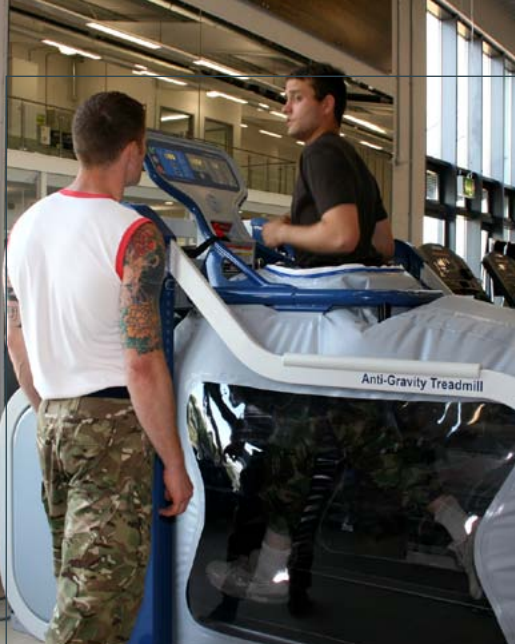
A recruit uses one of Parker Hall's anti-gravity treadmills. This equipment controls air pressure in a chamber to gently lift the user and reduce the impact of running on the feet and legs
