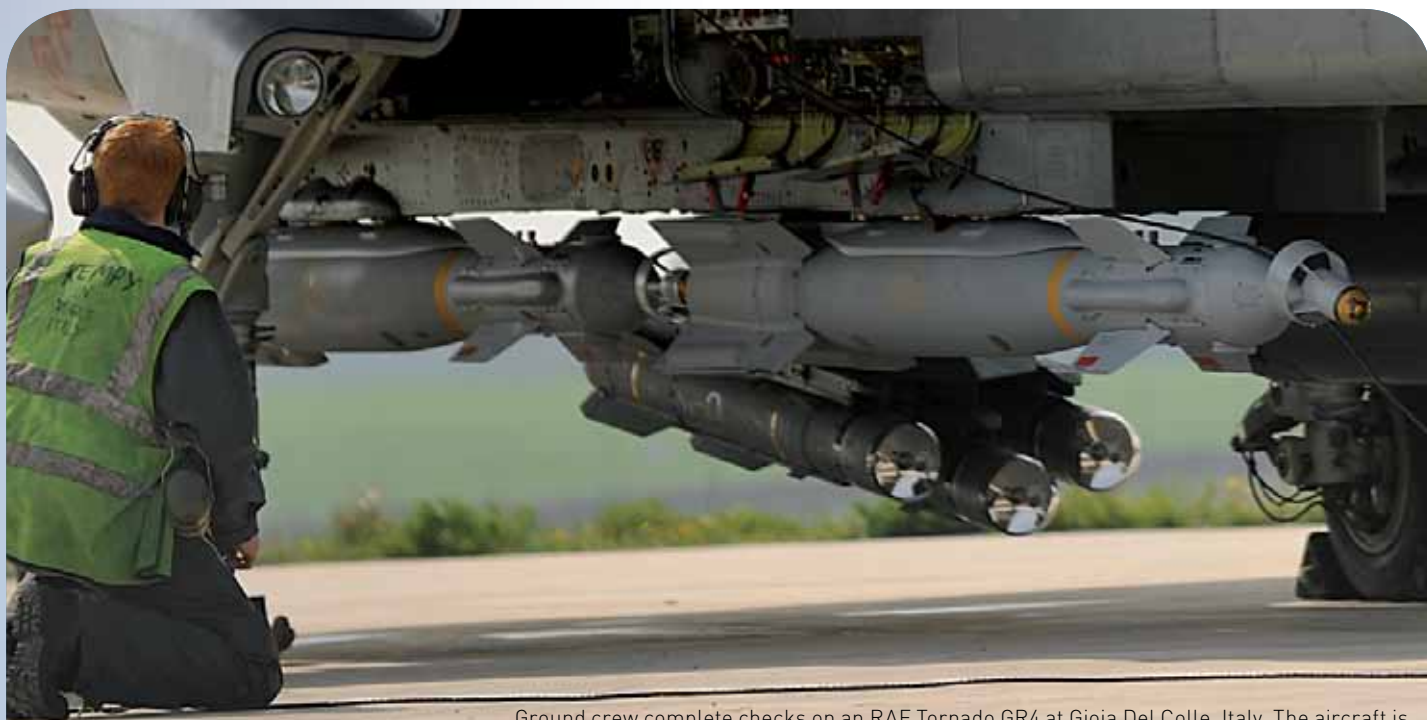
Ground crew complete checks on an RAF Tornado GR4 at Gioia Del Colle, Italy. The aircraft is armed with Paveway bombs and Brimstone missiles
