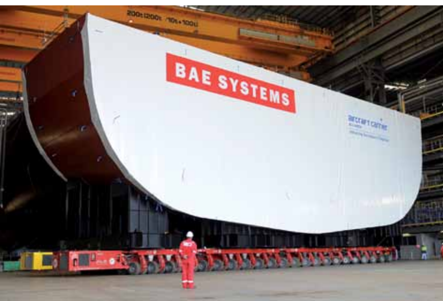
Rollout: one of the rings for Lower Block 05 of Queen Elizabeth is rolled out towards the barge at Portsmouth
