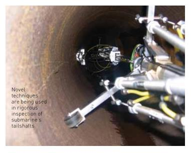
The tailshaft is now inspected from inside the tailshaft bore, using advanced NDT technology to penetrate the wall thickness and identify defects on the external surface from within.
