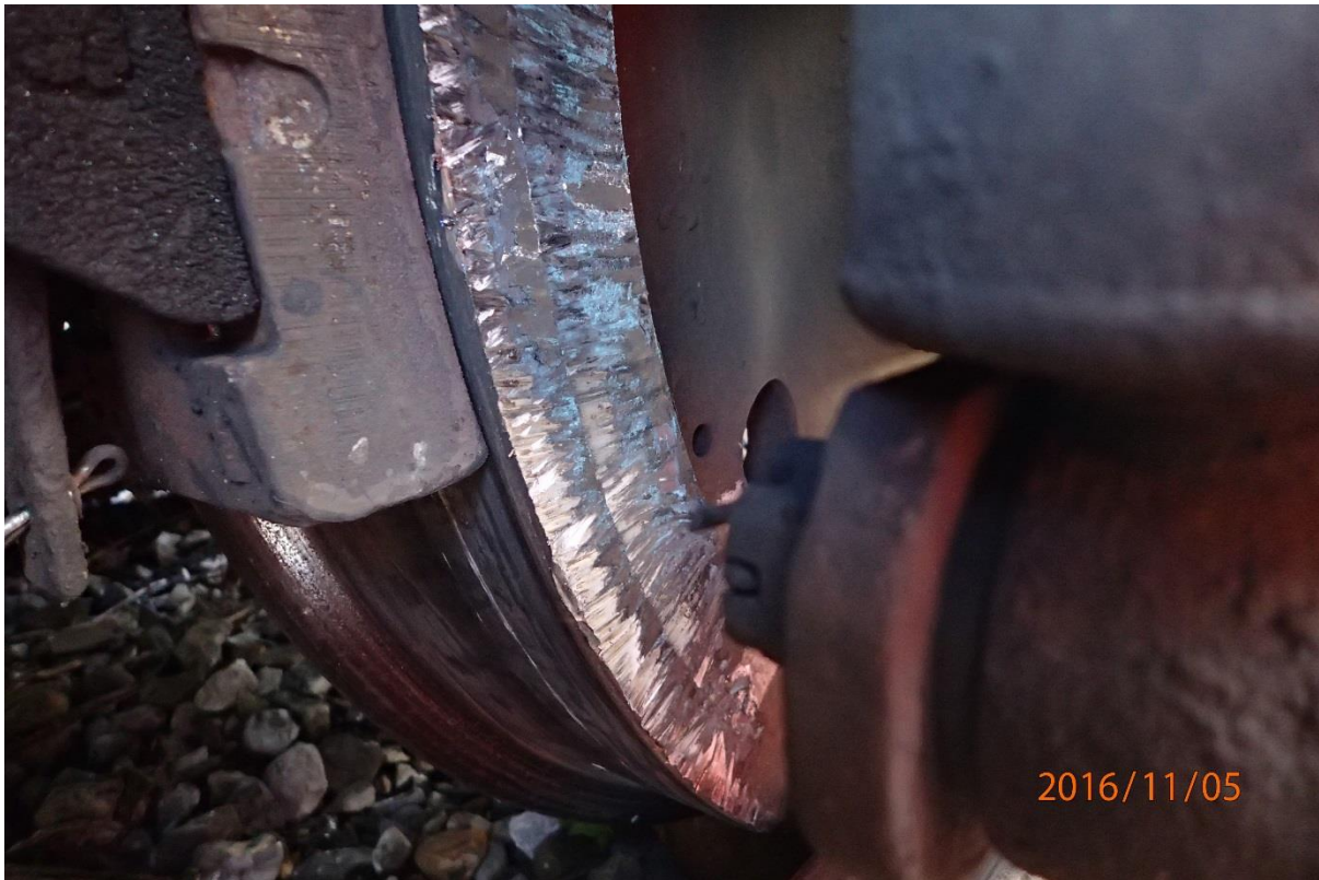
Significant bruising on the field face of the right-hand derailed wheels
