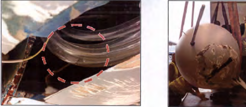
Figure 19 - WK031 Nose and Kollsman Pitot Probe Damage and Fluid found in Pipes
